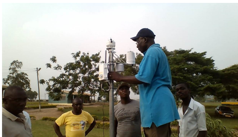
Plate 1: Staff from the Ghana Meteorological Agency installing a TAHMO Generation 2 Weather station in Ghana
