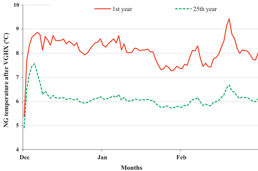
Fig. 8. NG temperature at the exit of the shell and tube heat exchanger.
