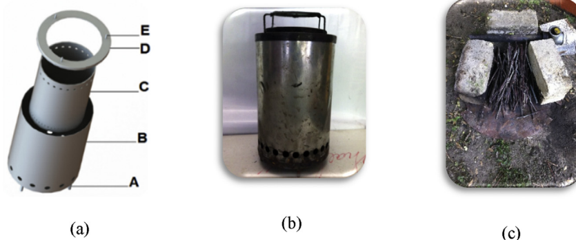
Fig. 1. View of the ICS (a and b) and the TCS (c). A) The outer cylinder legs. B) The outer cylinder. C) The inner cylinder. D) The outer and inner cylinder coupling. E) Connector bolt to air control top door.
