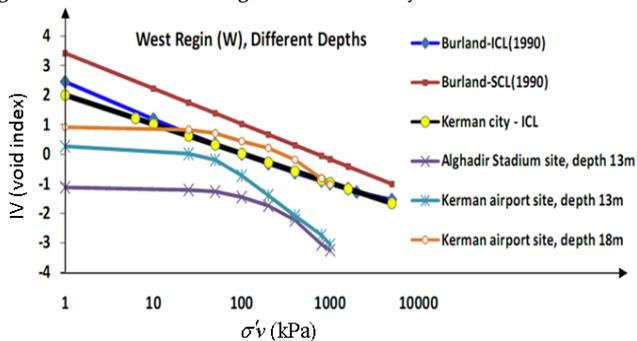
Fig. 9. Comparison of consolidation curves to Kerman-ICL in the western region at different depths.
