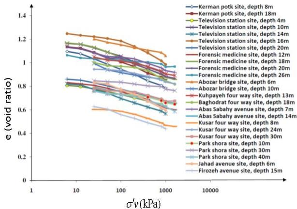
Fig. 3. Kerman-ICL in the e-Log( $\sigma'_v$ ) space.
