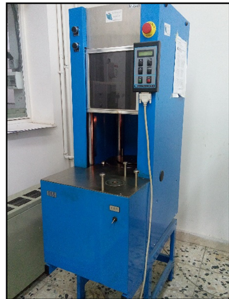
Fig. 4. The Superpave Gyratory Compactor device used for the mixture compaction purpose.
