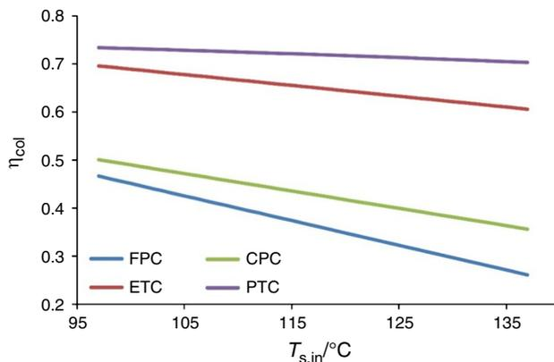
**Fig. 13** The efficiency of collectors as a function of heat source temperature level [52]. Reprinted with permission from Elsevier
