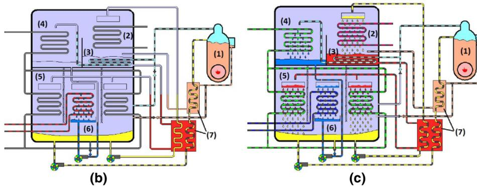
1-gas boiler (high pressure generator), 2-low pressure generator for single effect circulation, 3-low pressure generator for double effect circulation, 4-condensator, 5-absorber, 6-evaporator, 7-solution heat exchanger
