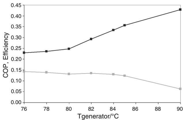
**Fig. 5** Variations of global efficiency (■) and heat pump COP (▲) versus the generator temperature [34]. Reprinted with permission from Elsevier
