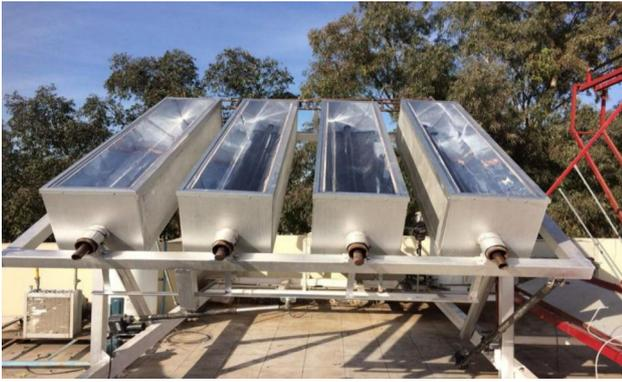
**Fig. 15** A photograph of the test section (compound parabolic concentrators with concentric tube absorber) studied by Acuña et al. [53]. Reprinted with permission from Elsevier
