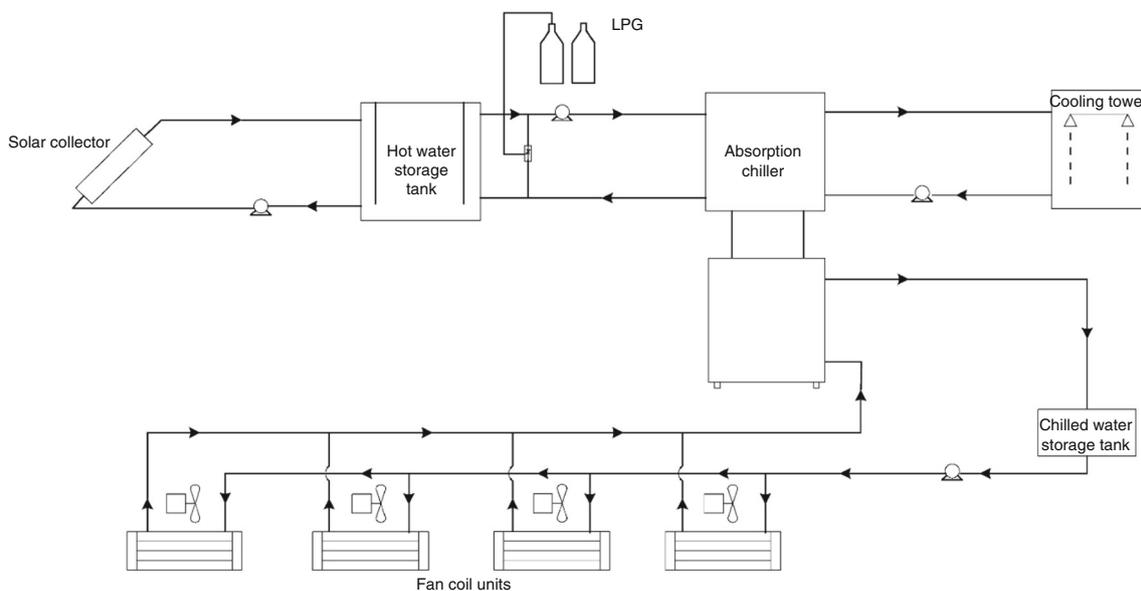
**Fig. 3** Schematic of the solar-powered single-effect absorption chiller studied by Pongtornkulpanich et al. [29]. Reprinted with permission from Elsevier
