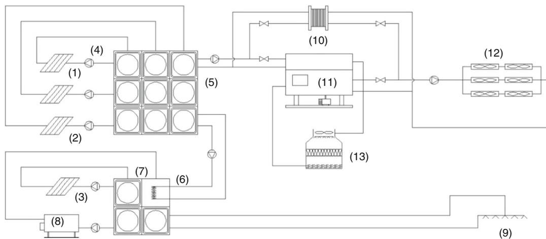
(1) Evacuated tube gravity heat pipe solar collector, (2) Evacuated tube horizontal heat pipe solar collector, (3) Evacuated glass tube solar collector, (4) Pump, (5) Water tank for air conditioning, (6) Cooper pipe heat exchanger, (7) Hotel hot water tank, (8) Auxiliary boiler, (9) Hot water use, (10) Plate heat exchanger, (11) Absorption chiller, (12) Fan coil, (13) Cooling tower
