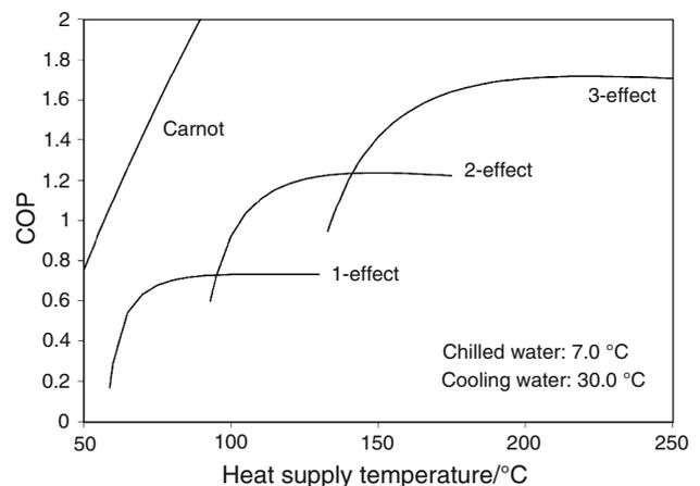
**Fig. 1** Variation of COP as a function of solar heat supply temperature for various LiBr–H<sub>2</sub>O absorption chiller types [54]. Reprinted with permission from Elsevier
