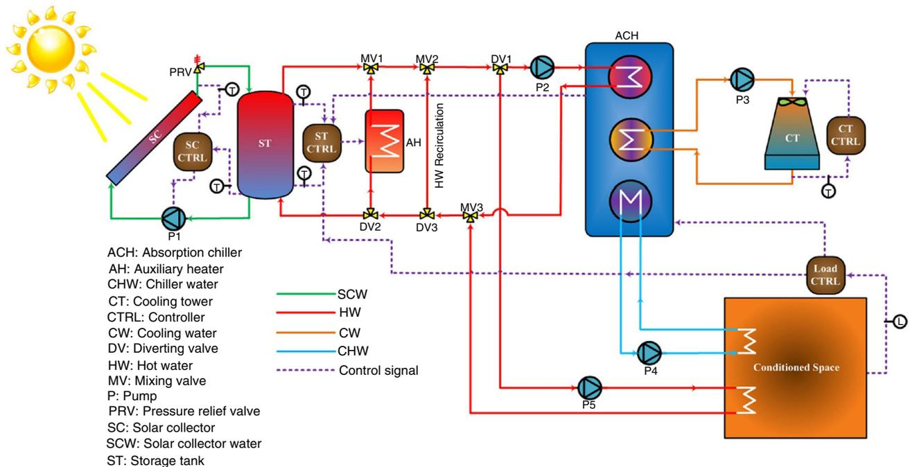
**Fig. 8** Schematic of an SHC absorption chiller layout [36]. Reprinted with permission from Elsevier
