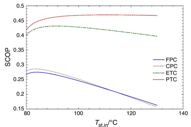
**Fig. 14** Variation of SCOP against heat source temperature for a cooling system pair with various collector types [59]. Reprinted with permission from Springer Nature
