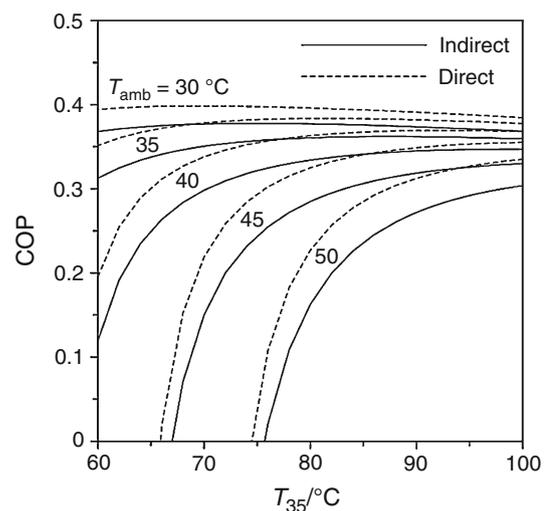
Fig. 10 The effects of ambient temperature on the performance of air-cooled LiBr/H<sub>2</sub>O absorption chillers (half-effect) [48]. Reprinted with permission from Elsevier
