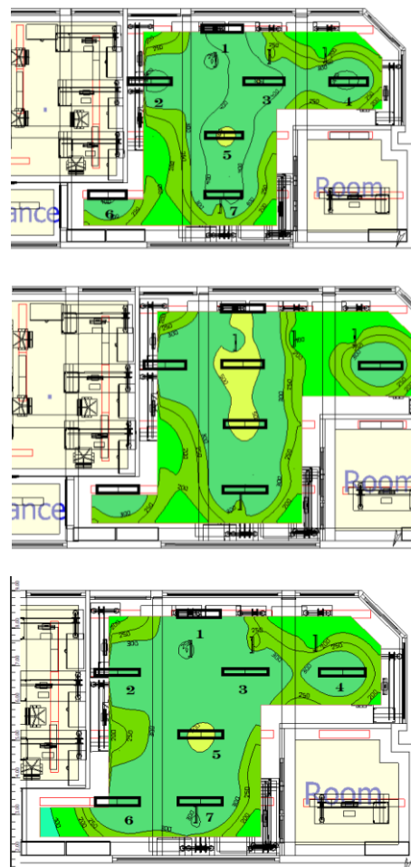
Fig. 6: Position of LEDs in best lighting scenarios, islanded mode
