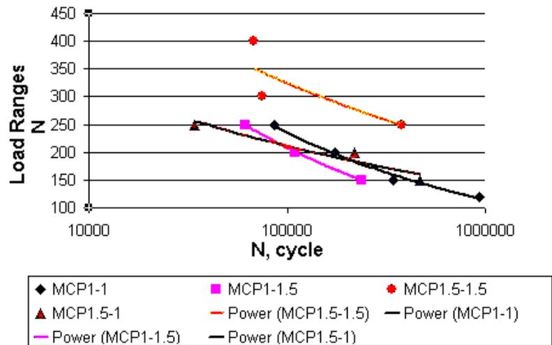
Figure 10: Result of load versus fatigue life of MCP spot weld specimens
