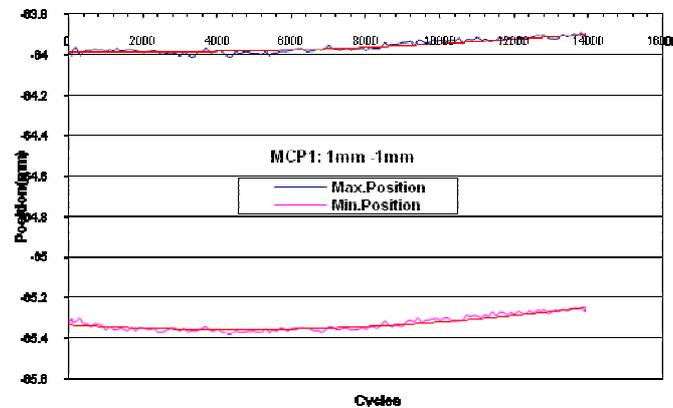
**Figure 22:** The displacement versus the number of loading cycles curve for MCP : 1mm-1mm specimen
