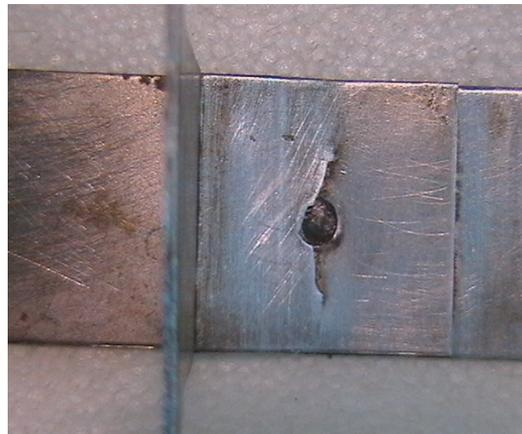
**c: manner of crack growth in L-sheet with 1.0mm thickness**
