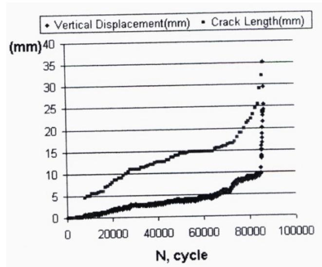
**Figure 17:** Comparison between the crack length and vertical displacement curves for MCP 10-10-4 specimen
