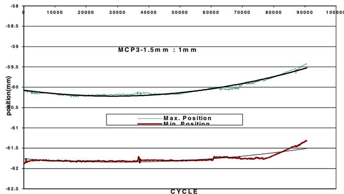
**Figure 21:** The displacement versus the number of loading cycles curve for MCP : 1mm-1.5mm specimen
