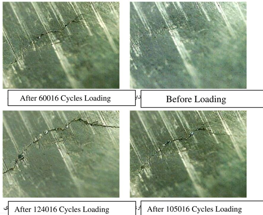
Figure 11: Crack growth images in MCP 10-10-4 specimen, during loading.
