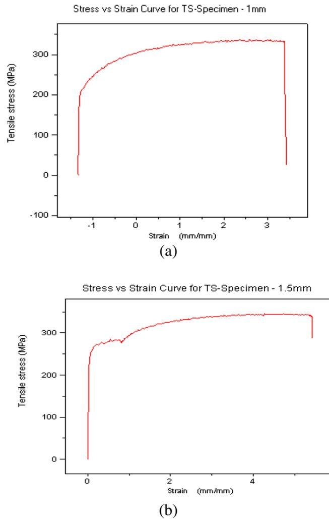
**Figure 5:** Stress-strain curves for spot weld sheets in uni-axial tensile test
