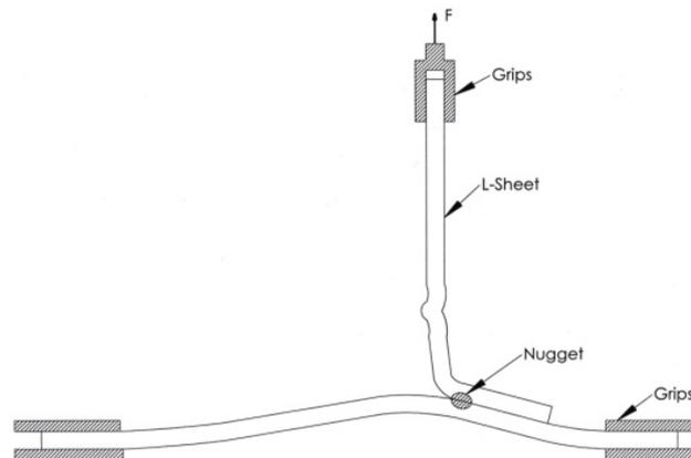
**Figure 3:** Tensile test for determining the tensile strength of nugget.
