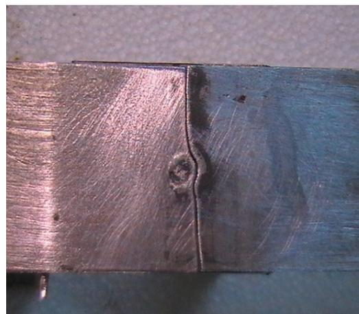
**a: manner of crack growth in straight sheet with 1.0 mm thickness**
