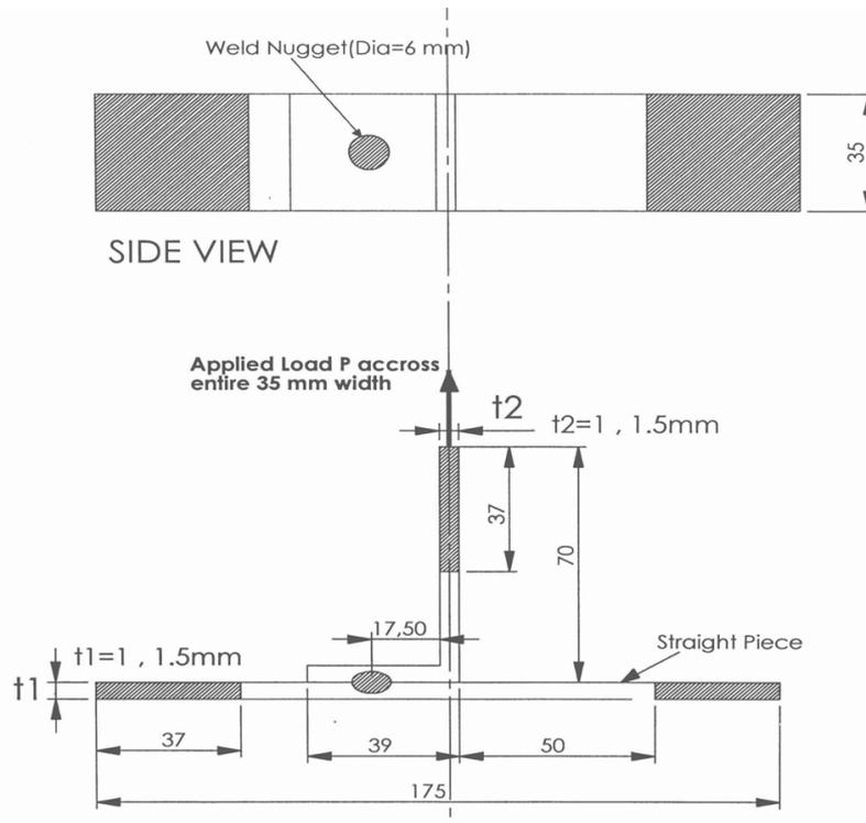
**Figure 1:** Geometry and dimensions of spot weld specimens
