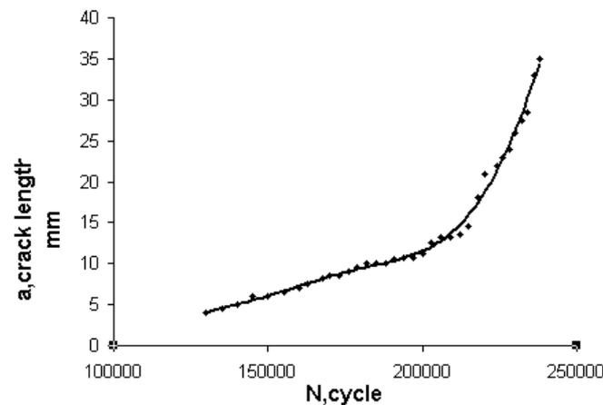
**Figure 15:**Crack length versus the number of cycle curve for specimens MCP10-15-1
