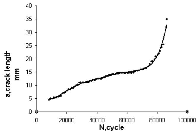
**Figure 14:**Crack length versus the number of cycle curve for specimens MCP10-10-4
