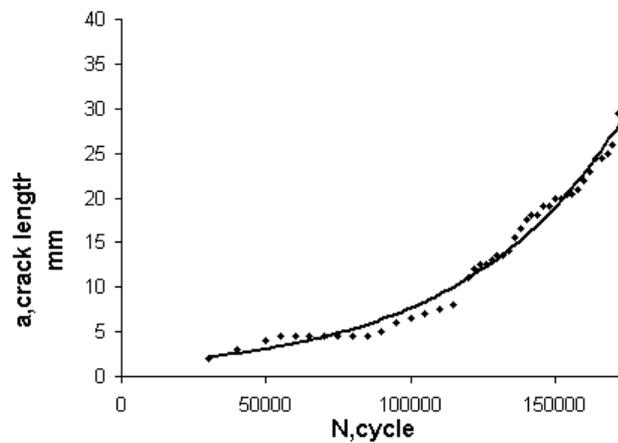
**Figure 13:** Crack length versus the number of cycle curve for specimen MCP 10-10-3
