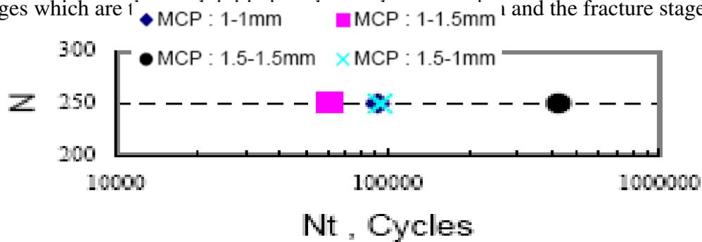
**Figure 9:** Results of load versus fatigue life of spot weld specimens in  $F_{max}=250N$
