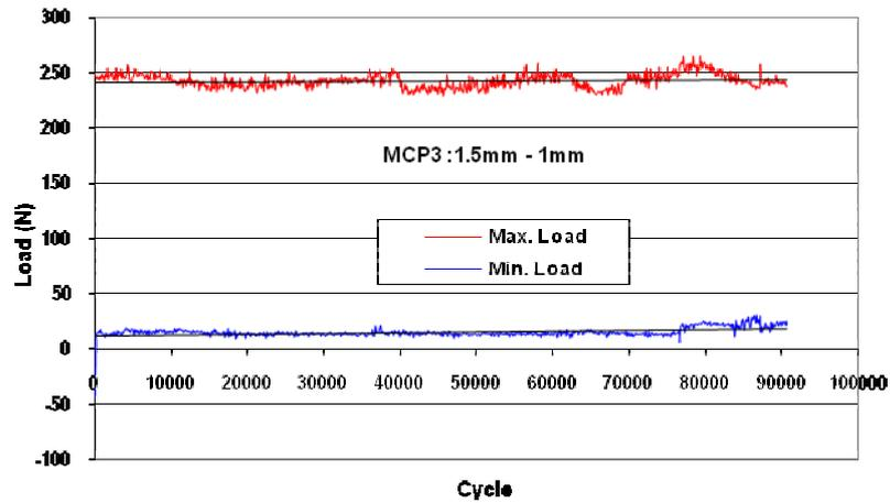
**Figure 18:** The load versus the number of loading cycles curve for for MCP : 1.5mm-1.5mm specimen
