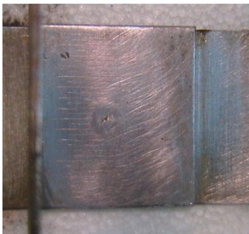
**b: in L-sheets with 1.5 mm thickness, there is not crack**
