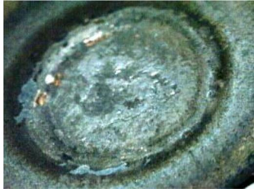
**Figure 2:** Spot weld section on the surface of specimen
