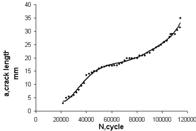
**Figure 16:**Crack length versus the number of cycle curvefor specimens MCP 10-15-3
