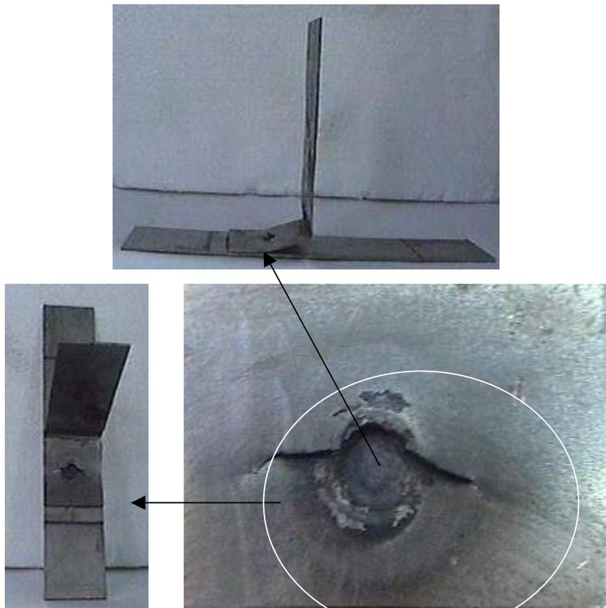
**Figure 25:** Location of initiation and propagation of a crack in a real specimen
