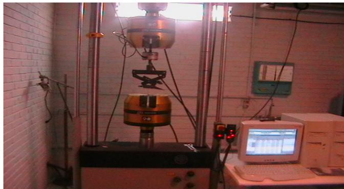
**Figure 6:** Apparatus set up of specimens on INSTRON 8802 Fatigue test machine
