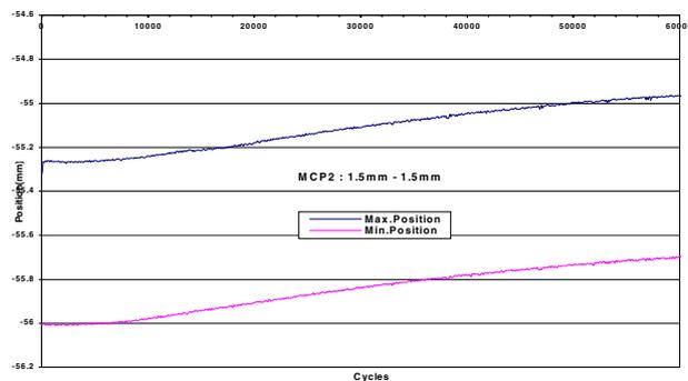
**Figure 19:** The displacement versus the number of loading cycles curve for MCP : 1.5mm-1.5mm specimen
