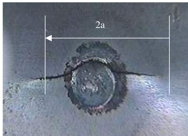
**Figure 8:** Crack in length 2a
