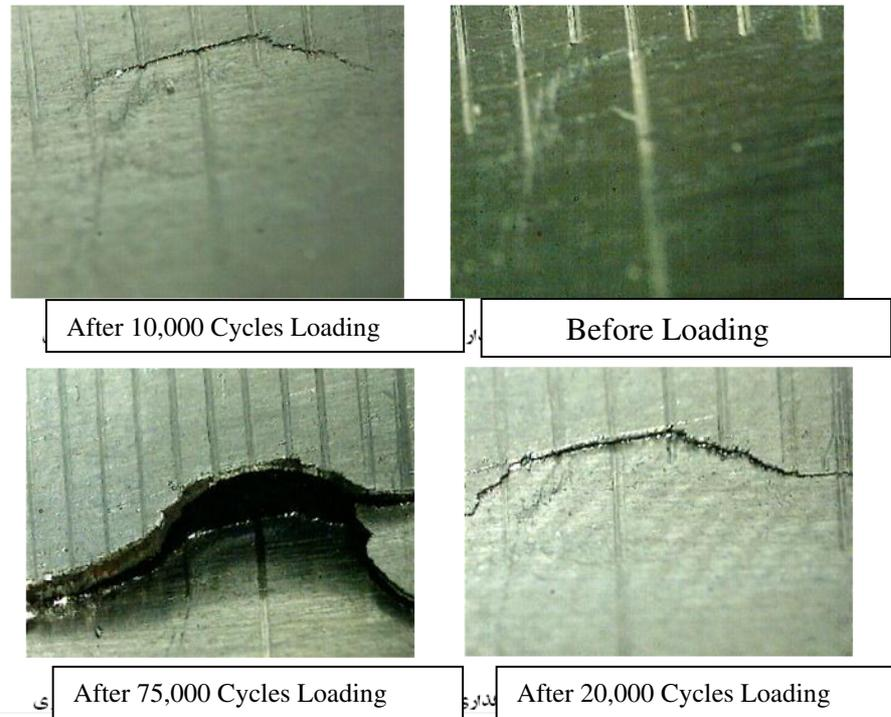
**Figure 12:** Crack growth images in MCP 10-15-1 specimen, during loading
