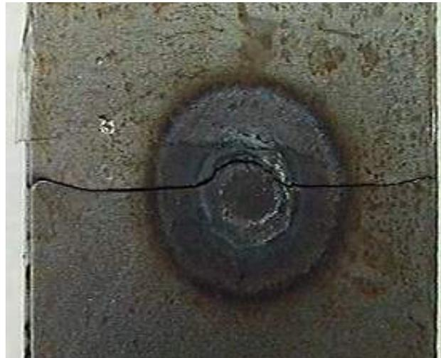
**Figure 7:** Complete fracture of a sheet
