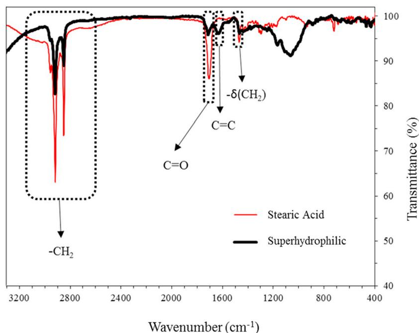
Fig. 2. FTIR spectra of superhydrophobic electrodeposited film and stearic acid powder. The resolution was set to  $4\text{ cm}^{-1}$  and the number of scans was 32.
