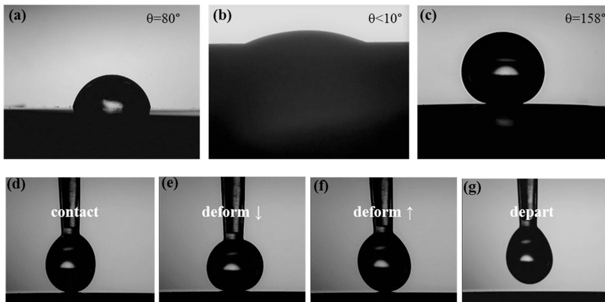
Fig. 3. Photographs of water droplets during the contact angle measurement on (a) bright Ni (b) hydrophilic and (c) superhydrophobic surfaces. (d–g) Steps showing the water droplet contacts the superhydrophobic surface, deforms during the approach, deforms during the departure, and finally departs the surface. The water droplet does not stick to the superhydrophobic surface and is easily detached.
