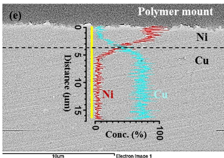
Fig. 1. (a–c) SEM surface morphology of the micro-nano structured electrodeposited film (e) Cross-sectional SEM images. The inset shows the EDS elemental line profile analysis along the yellow line. The interface between Cu substrate and Ni film is marked with a dashed line based on the EDS line profile results.
