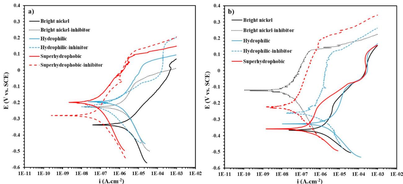
Fig. 4. The potentiodynamic polarization curves of bright, hydrophilic, and superhydrophobic electrodeposited Ni film in 3.5 wt% NaCl solutions with and without inhibitor (a) after 30 min (b) after 120 h immersion.
