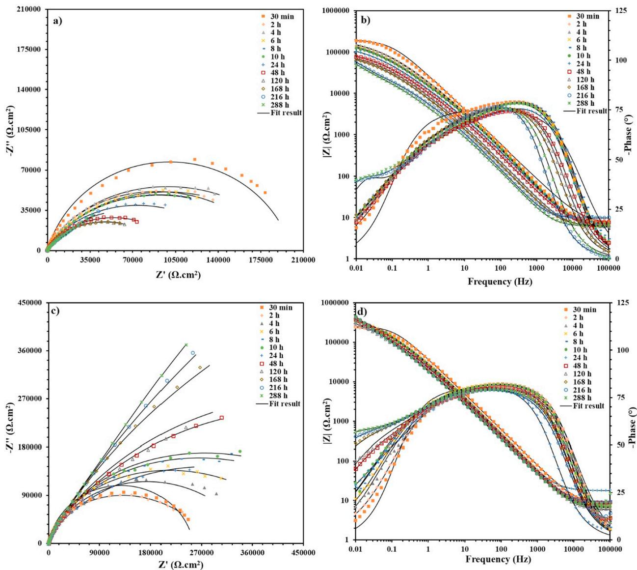
**Fig. 5.** EIS results for superhydrophobic Ni film without inhibitor (a) Nyquist and (b) Bode (resistance magnitude and phase angle) representation. (c) and (d) show the Nyquist and Bode results for the superhydrophobic sample with 0.2 g/L 4Mpy inhibitor in solution. EIS curves for different immersion times are presented with different symbols. Lines are fits to the experimental data (symbols).
