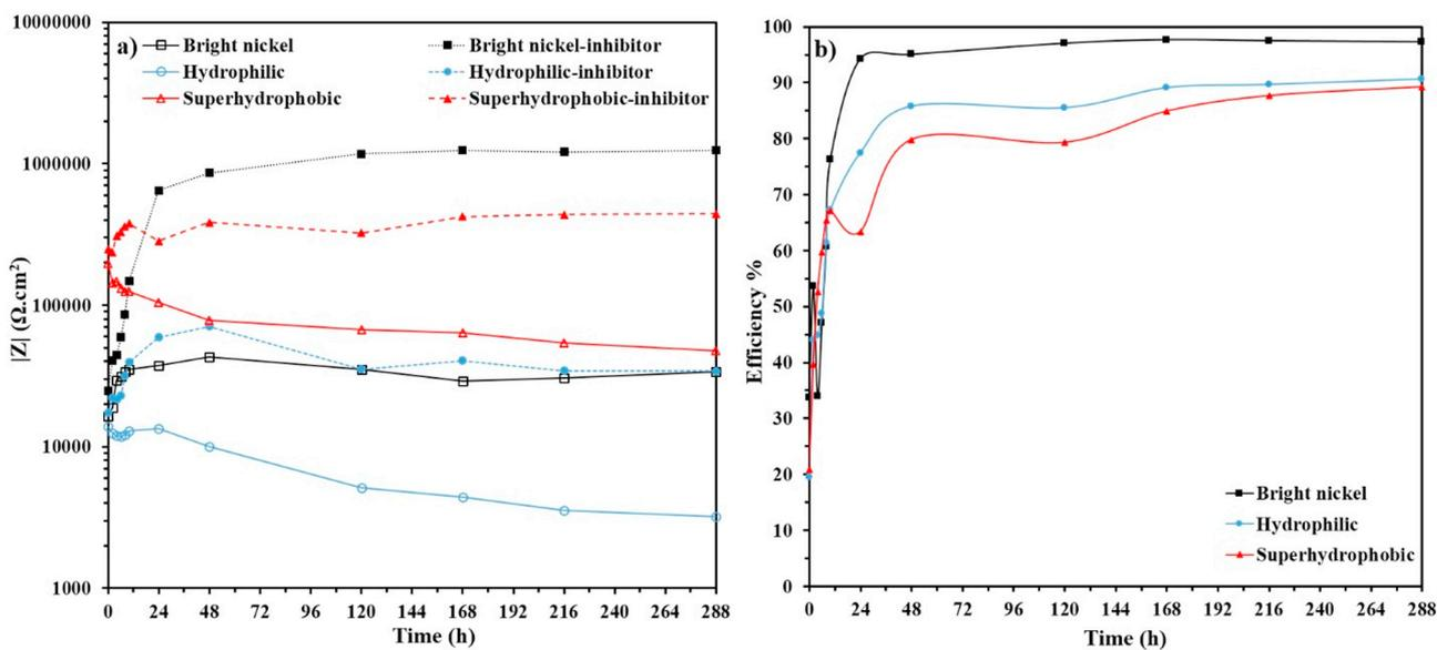
Fig. 9. Effect of immersion time on (a) absolute impedance module at 0.01 Hz and (b) corrosion inhibitor efficiency on bright, hydrophilic and superhydrophobic Ni surfaces immersed in 3.5 wt% NaCl solution. The lines connecting the symbols (experimental data) are guide to the eyes.
