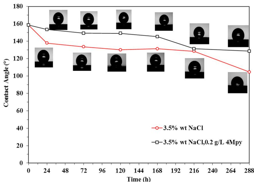
Fig. 10. Changes of water CA of the superhydrophobic surface with the immersion time in 3.5 wt% NaCl solution with and without  $0.2 \text{ g} \cdot \text{L}^{-1}$  4Mpy. The lines connecting the symbols (experimental data) are guide to the eyes.
