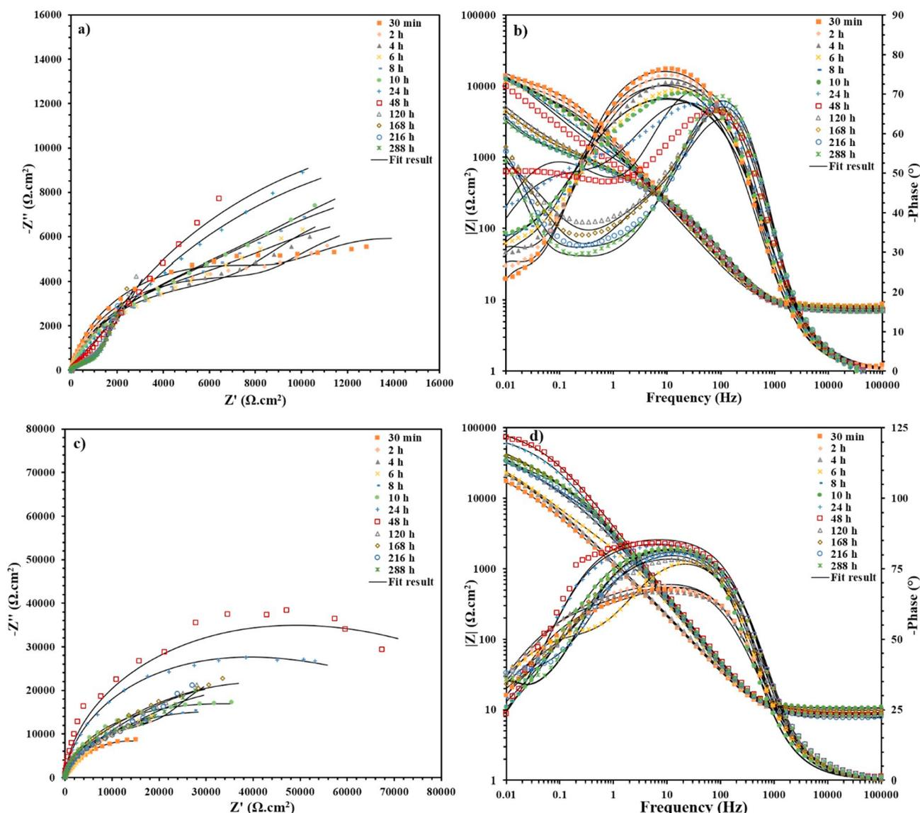
**Fig. 6.** EIS results for hydrophilic Ni film without inhibitor (a) Nyquist and (b) Bode (resistance magnitude and phase angle) representation. (c) and (d) show the Nyquist and Bode results for the superhydrophobic sample with 0.2 g/L 4Mpy inhibitor in solution. EIS curves for different immersion times are presented with different symbols. Lines are fits to the experimental data (symbols).
