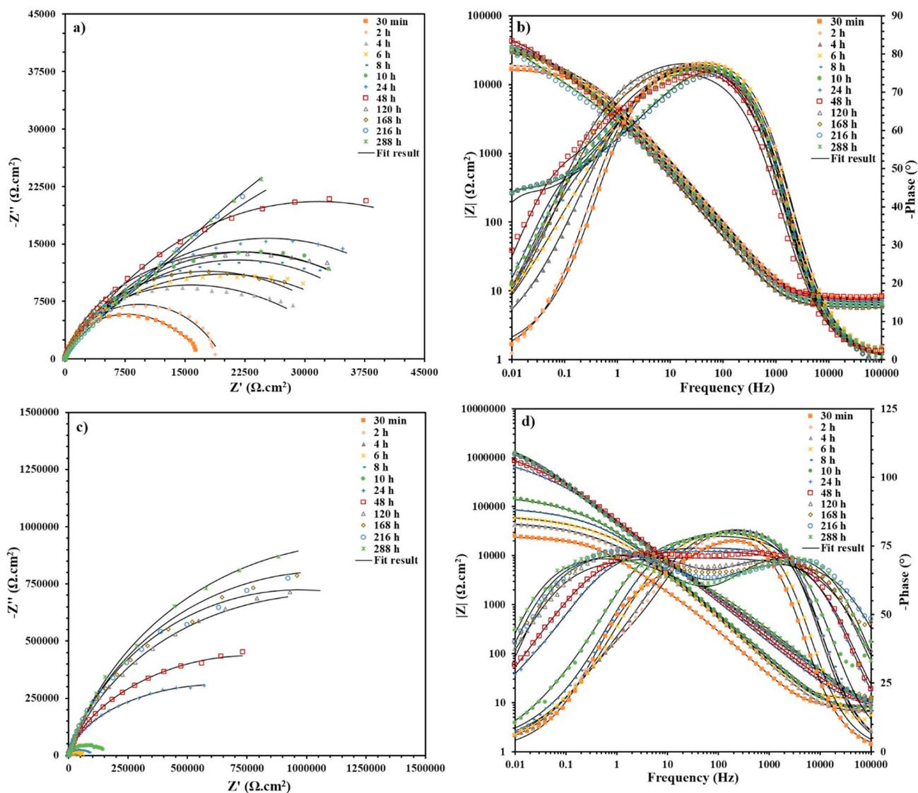
Fig. 7. EIS results for bright Ni film without inhibitor (a) Nyquist and (b) Bode (resistance magnitude and phase angle) representation. (c) and (d) show the Nyquist and Bode results for the superhydrophobic sample with 0.2 g/L 4Mpy inhibitor in solution. EIS curves for different immersion times are presented with different symbols. Lines are fits to the experimental data (symbols).
