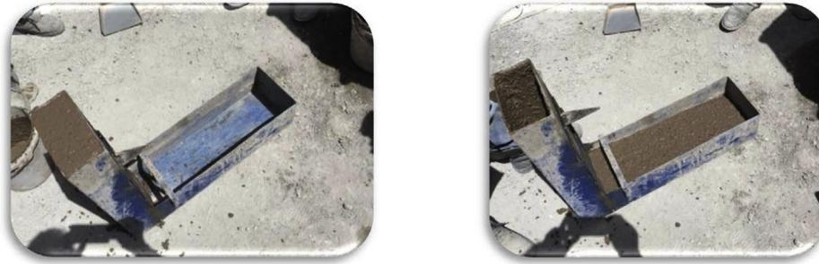
Fig. 7. L-box test of B4 sample before and after opening the gate.
