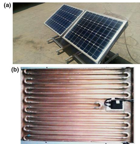
**Fig. 1** A view of the **a** PV and PVT modules and **b** serpentine tube collector
