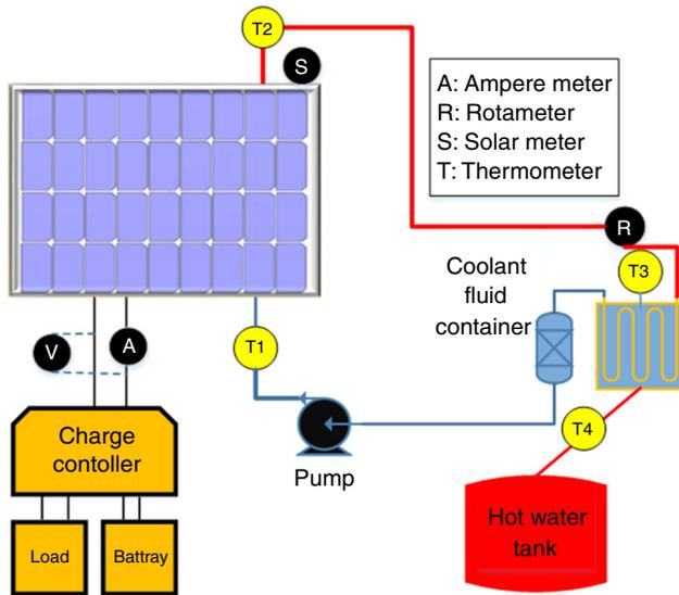
**Fig. 2** Serpentine tube collector attached to the backside of the photovoltaic module
