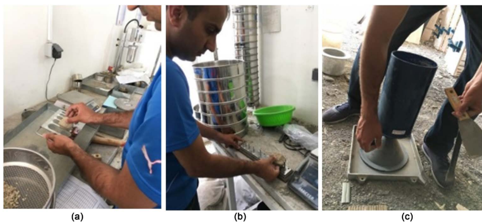
Figure 3. Tests steps and devices: (a) Flakiness test; (b) Elongation test; (c) Sand bottle method.
