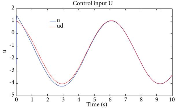
**Figure 8.** Control input  $u$  and nominal input  $u_d$ .
