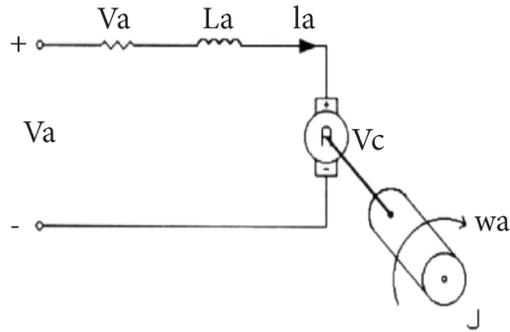
Figure 9. Electrical circuit of the DC motor.
