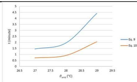
**Figure 6.** The chart of fan-coil  $t - \vartheta_{amb}$  for room 2.
