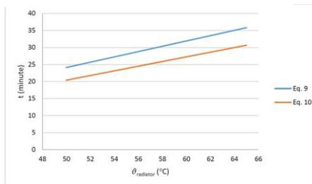
**Figure 8.** The chart of 11 blades radiator  $t - \vartheta_{radiator}$  for room 2.
