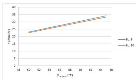
**Figure 9.** The chart of 12 blades radiator  $t - \vartheta_{radiator}$  for room 2.
