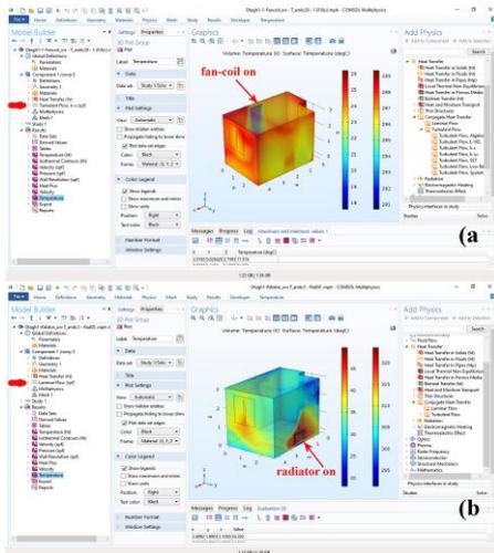
**Figure 2.** (a) turbulent flow (for fan-coil); and (b) laminar flow (for radiator) (room 1) [3, 6].
