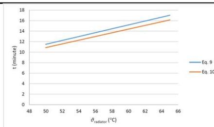
**Figure 10.** The chart of  $t - \vartheta_{radiator}$  for room 2 when both radiators are on.
