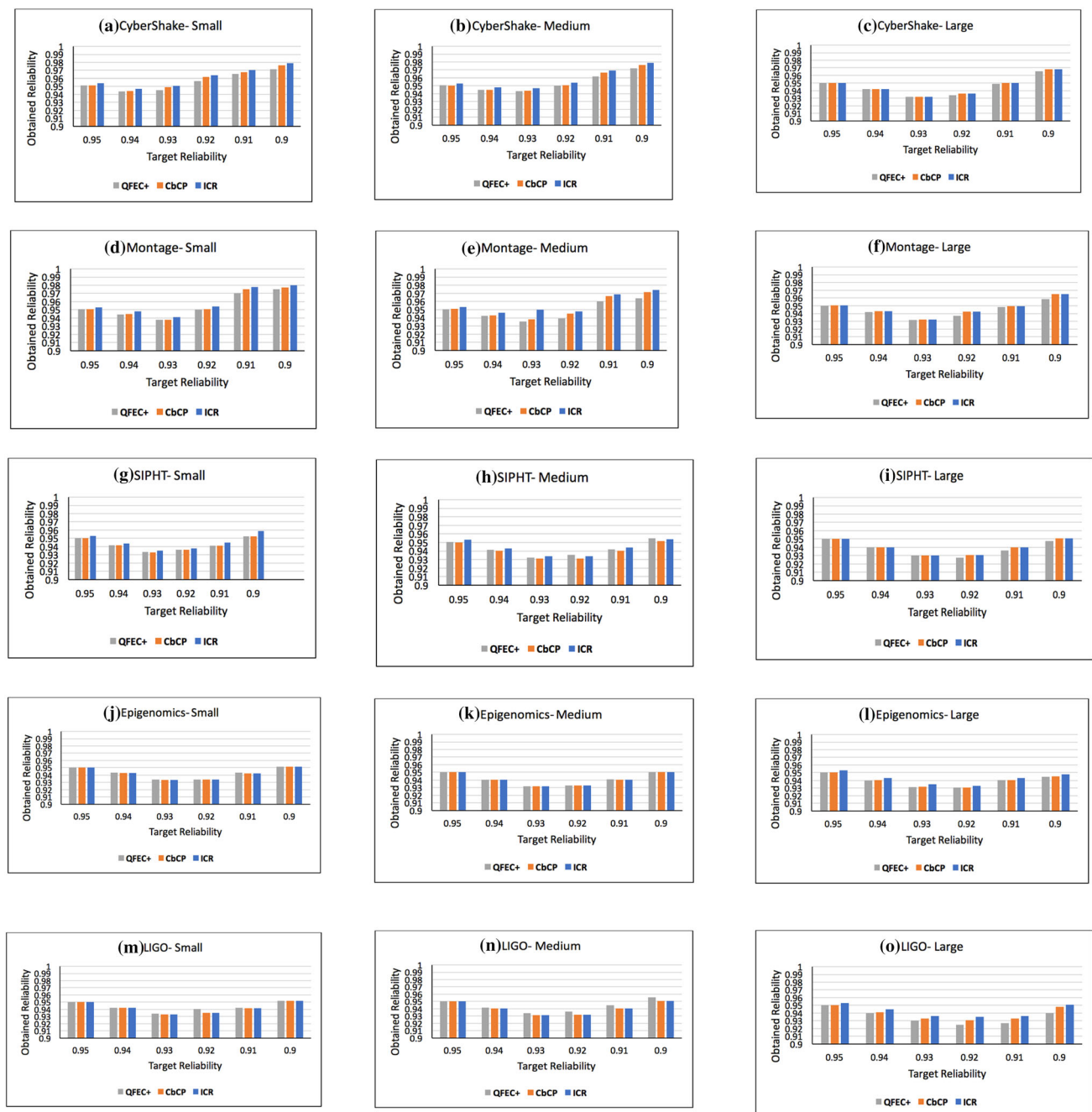
Fig. 6 Obtained Reliability of scheduling workflows with the ICR, CbCP and QFEC+ algorithms
