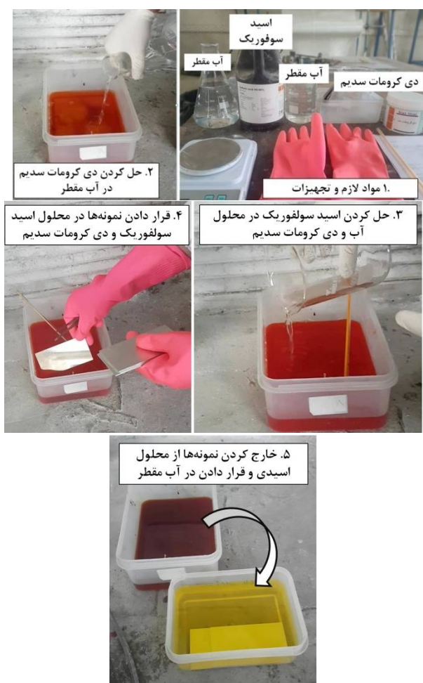
Fig. 3 Surface preparation method of the metallic surfaces
