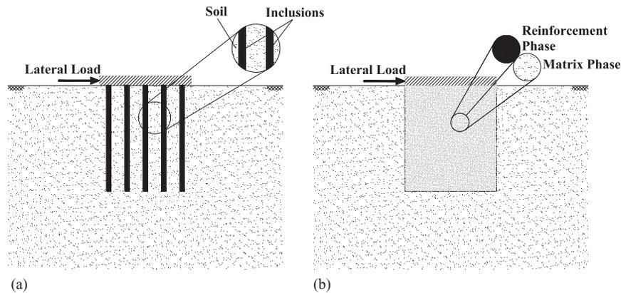
**Fig. 1.** Schematics of a laterally loaded pile group: (a) in a discrete form; and (b) as a two-phase material.
