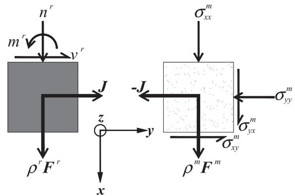
**Fig. 2.** Stress components and force vectors in a two-phase system. Signs are positive.
