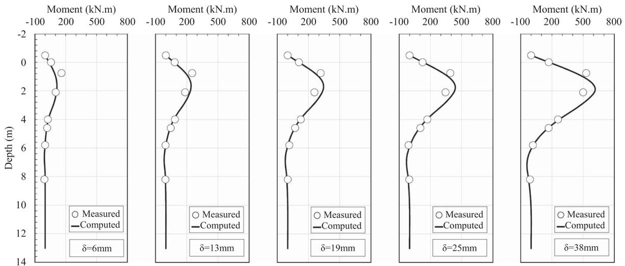
**Fig. 10.** Comparison of bending moments profiles measured in a full-scale test on a  $3 \times 5$  pile group (Walsh 2005) and computed bending moments profiles by using the proposed method for different pile-head displacements.
