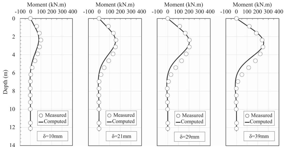
**Fig. 8.** Comparison of bending moments profiles measured in a full-scale test on a 3 × 3 pile group (Rollins et al. 2005) and computed bending moments profiles using the proposed method for different pile-head deflections.
