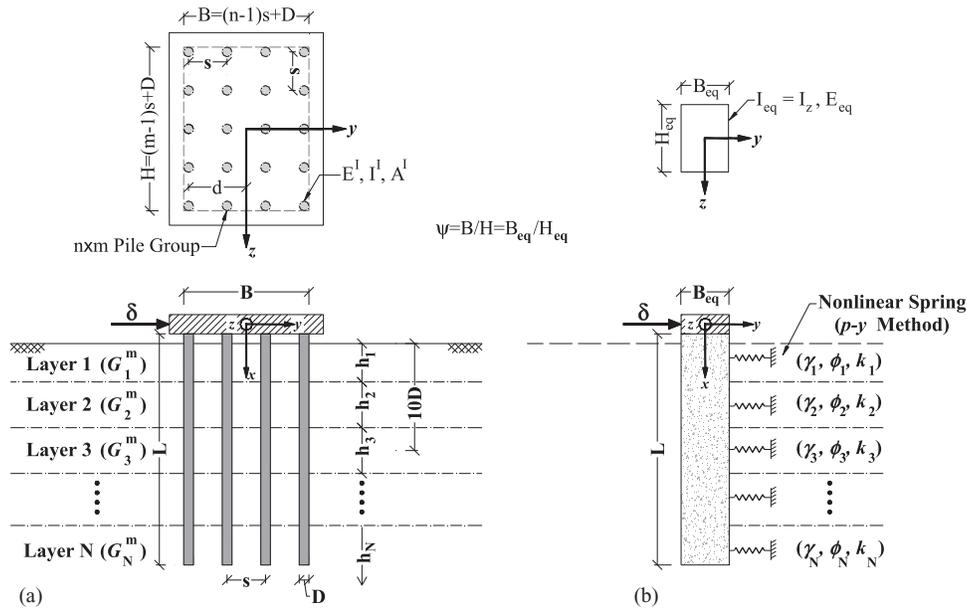
**Fig. 6.** A graphical scheme of the proposed hybrid approach for the analysis of a laterally loaded pile group located in a multilayered soil profile: (a) the pile group; and (b) the ESP.
