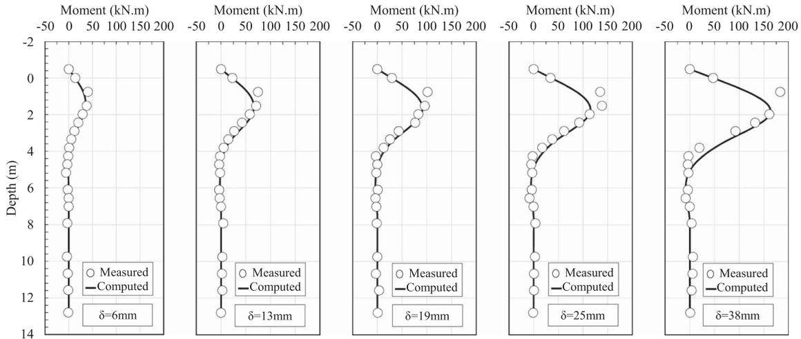
**Fig. 9.** Comparison of measured and computed bending moments versus depth at different pile-head deflections for the single pile test performed by Walsh (2005).
