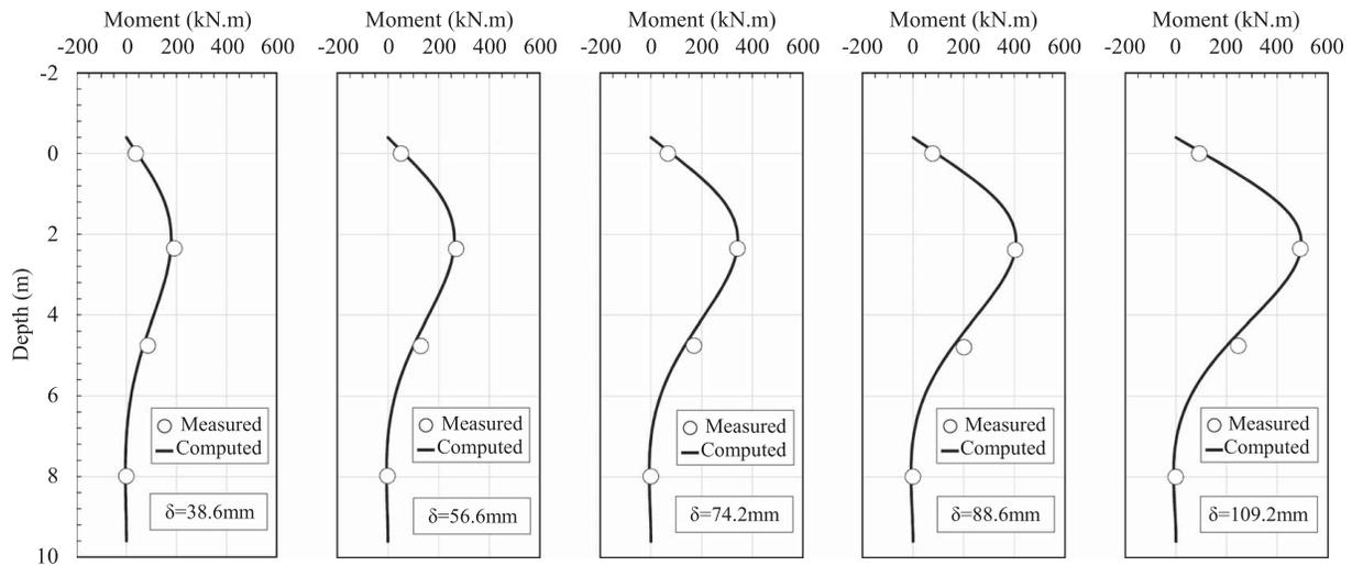
**Fig. 13.** Comparison of measured and computed bending moments versus depth at different pile-head deflection for the pile group test performed by Tobita et al. (2004) using the proposed method.
