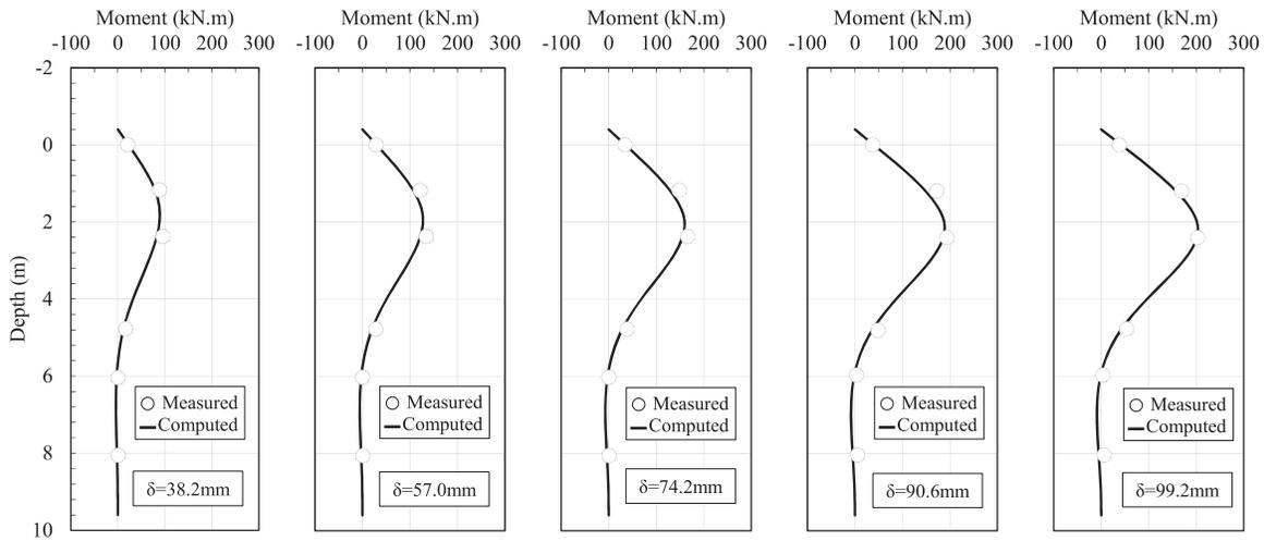
**Fig. 12.** Comparison of measured and computed bending moments versus depth at different pile-head deflection for the single pile test performed by Tobita et al. (2004).
