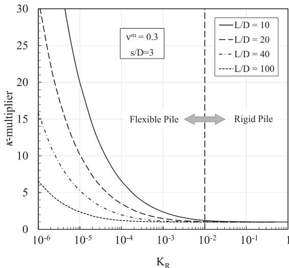
**Fig. 15.**  $\kappa$ -multiplier versus pile flexibility factor ( $K_R$ ) for various  $L/D$  with  $v^m = 0.3$  and  $s/D = 3$ .
