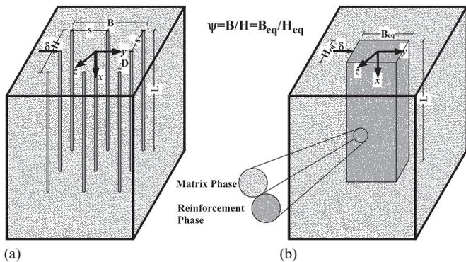
**Fig. 3.** Three-dimensional view of (a) a pile group; and (b) ESP as a two-phase system.
