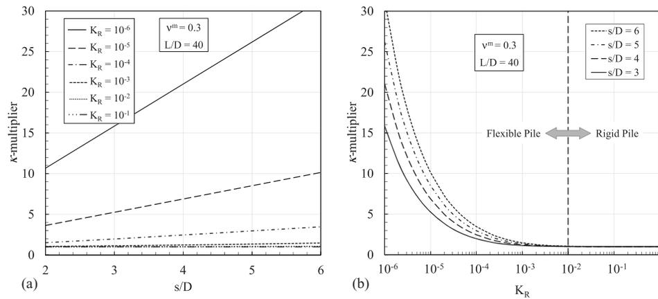
**Fig. 14.** Variation of  $\kappa$ -multiplier versus: (a) pile spacing ( $s/D$ ); and (b) pile flexibility factor ( $K_R$ ) for  $v^m = 0.3$  and  $L/D = 40$ .
