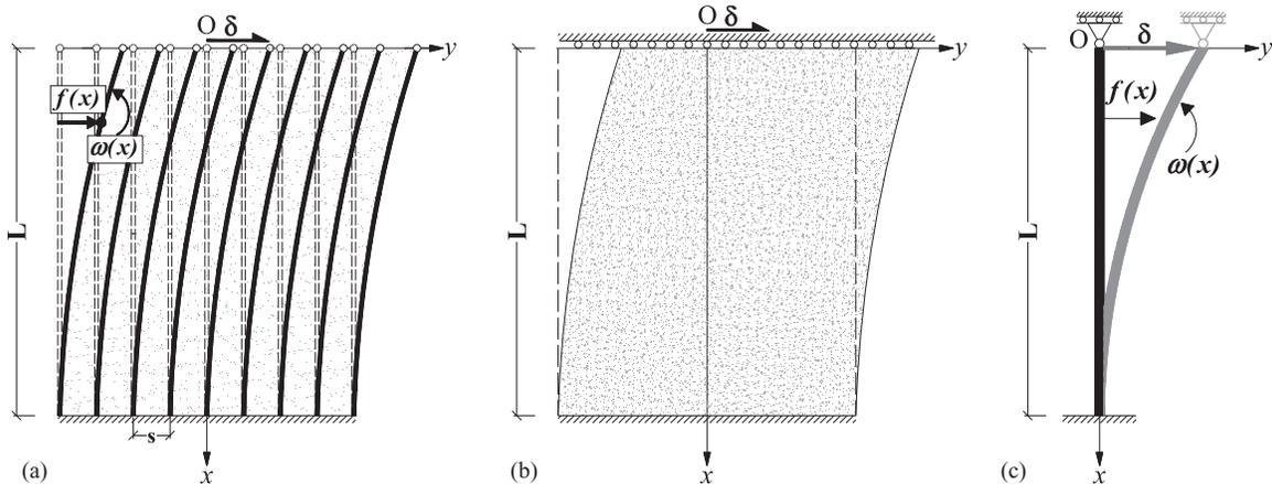
**Fig. 4.** Presentation of an elastic shear-loaded reinforced-soil layer with specific boundary conditions in the form of (a) discrete view; (b) two-phase system; and (c) a beam called as ESP, whose properties are equivalent to the pile group as a two-phase system.
