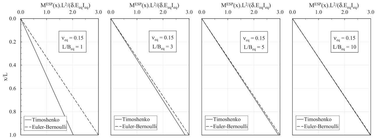
**Fig. 5.** Variations of dimensionless bending moment function of a laterally loaded ESP with normalized length considering Euler–Bernoulli and Timoshenko beam theories.
