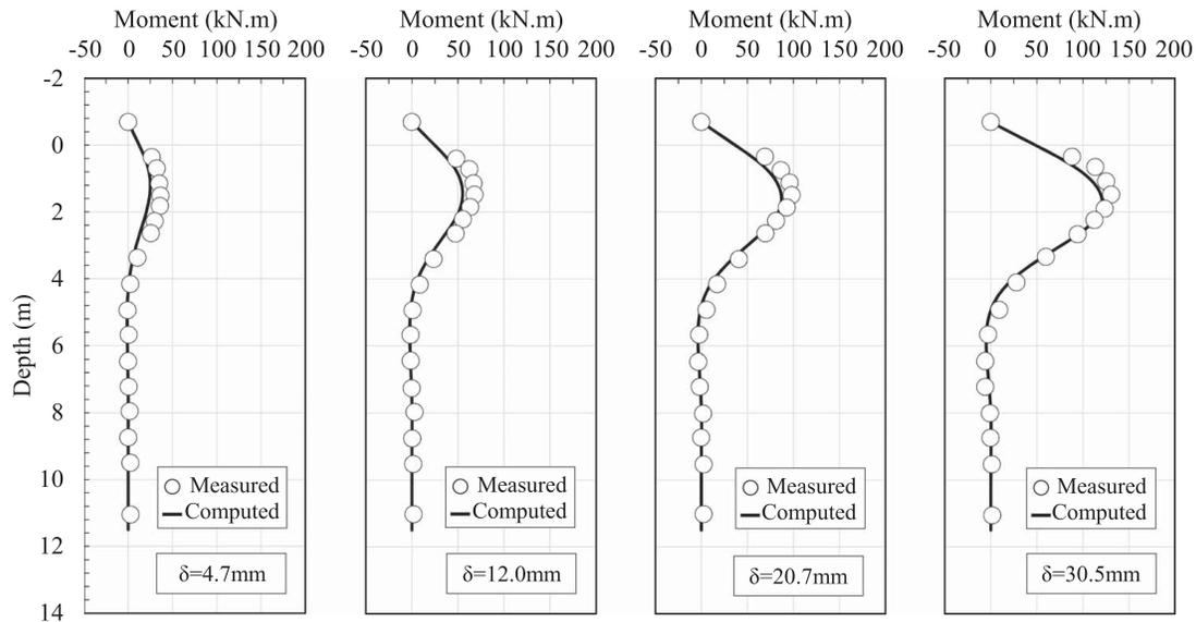
**Fig. 7.** Comparison of measured and computed bending moments versus depth at different pile-head deflections for the single pile test performed by Rollins et al. (2005).
