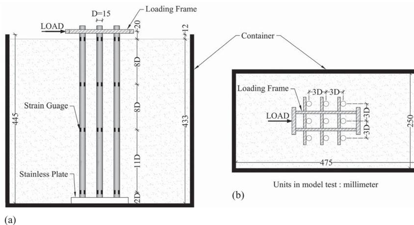
Fig. 11. Model setup in the centrifuge tests for static loading: (a) section view; and (b) plan view (Tobita et al. 2004).
