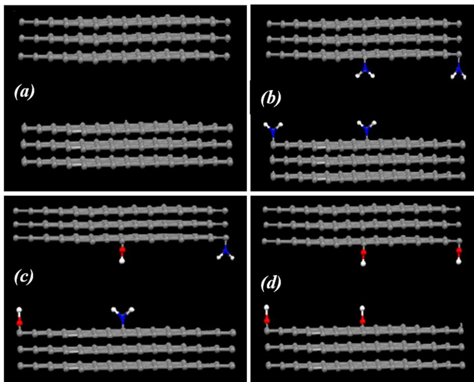
Fig. 2. Activated carbon model of (a) three-layer graphite, (b) graphite wall with amine groups, (c) graphite wall with hydroxyl groups, and (d) graphite wall with amine and hydroxyl groups.
