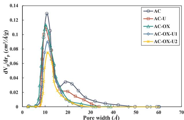
Fig. 5. Pore size distribution for the activated samples of: ○, AC; □, AC-U; △, AC-OX; ◇, AC-OX-U1; \*, AC-OX-U2.
