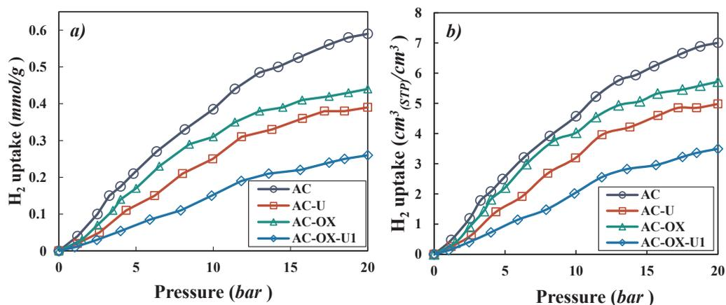
Fig. 8. H<sub>2</sub> adsorption isotherms for the activated samples of: ○, AC; □, AC-U; △, AC-OX; ◇, AC-OX-U1; \*, AC-OX-U2; at 298 K in a) gravimetric and b) volumetric calculation basis.
