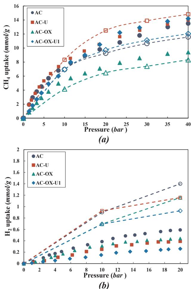
Fig. 12. Computed and measured adsorption isotherms of a)  $\text{CH}_4$  and b)  $\text{H}_2$  on activated carbons of: ●, AC; ■, AC-U; ▲, AC-OX; ◆, AC-OX-UI; with different functional groups at 298 K. Filled and empty symbols (with dotted lines) represent experiment and GCMC simulation data, respectively.
