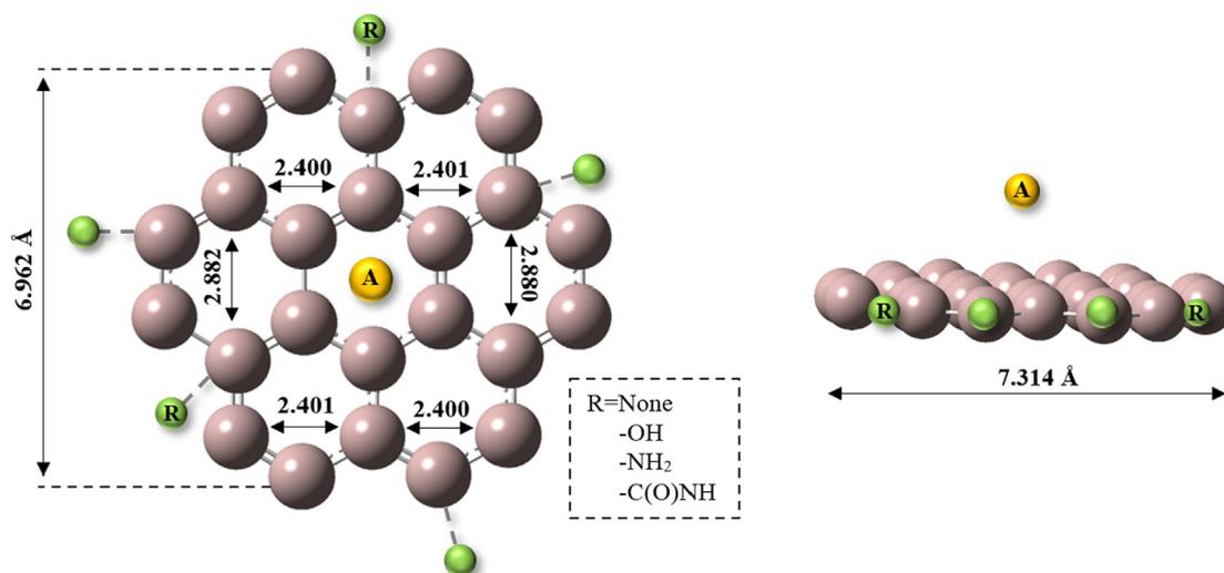
**Fig. 1.** Initial configurations of gas ( $\text{CH}_4$ ,  $\text{H}_2$ ) adsorption on edge-functionalised carbon basis unit. The top view (left) and side view (right) are illustrated. Nomenclature: A, adsorbate position above the centre of a benzene ring in basis unit; R, attached functional group. Colour Code: Gray Pink -Carbon, Green -R, Yellow -A.
