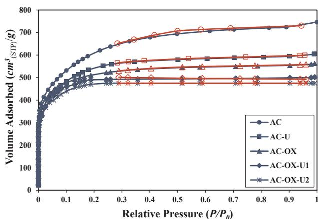
Fig. 4.  $N_2$  adsorption/desorption isotherms for activated coal-based samples of: ●, AC; ■, AC-U; ▲, AC-OX; ◆, AC-OX-U1; \*, AC-OX-U2. Filled and empty symbols represent the nitrogen adsorption and desorption, respectively.
