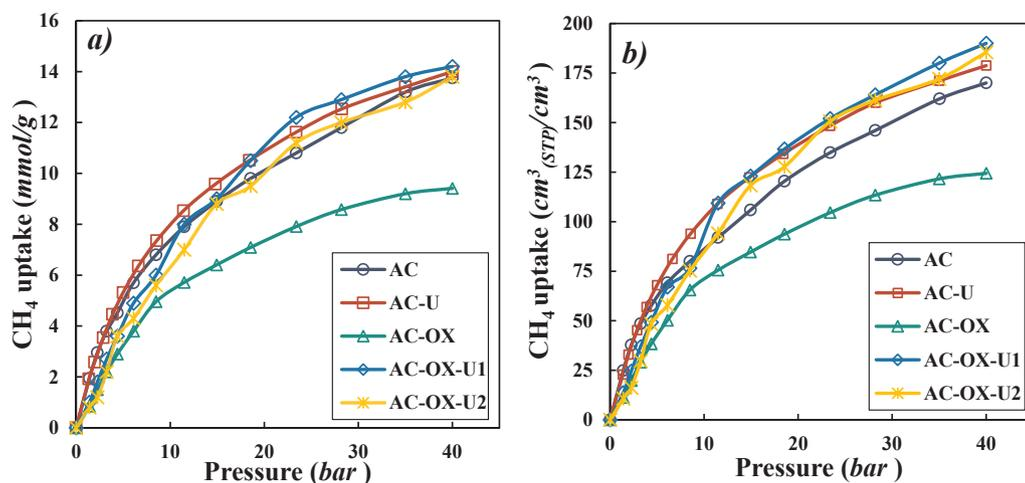
Fig. 7. Methane adsorption isotherms for the activated samples of: ○, AC; □, AC-U; △, AC-OX; ◇, AC-OX-U1; \*, AC-OX-U2; at 298 K in a) gravimetric and b) volumetric calculation basis.
