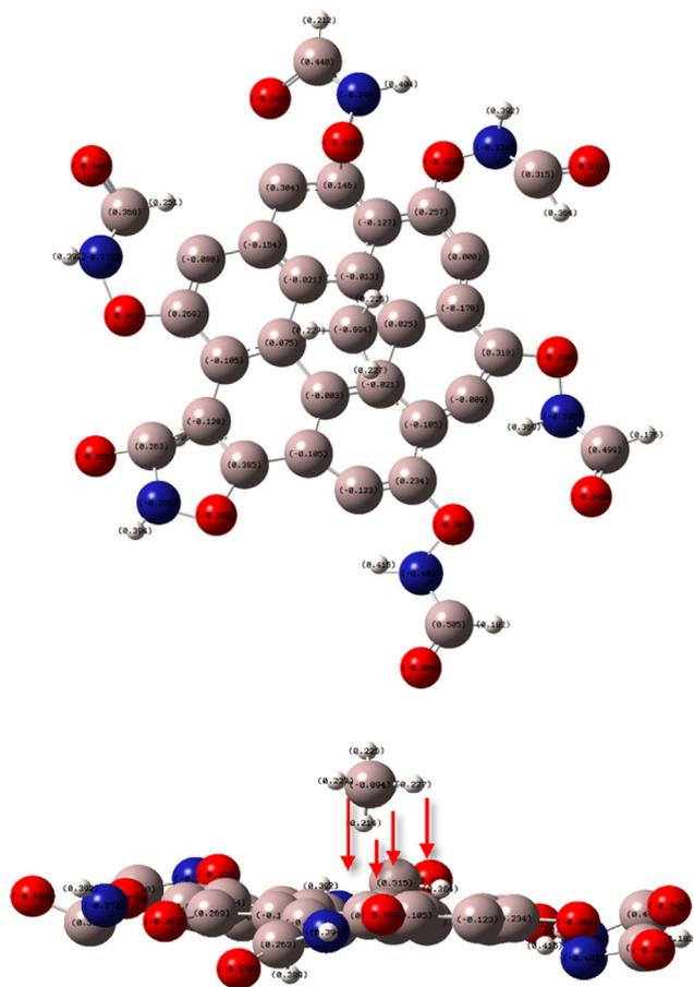
Fig. 10. Schematic display of the interaction between the adsorbate ( $\text{CH}_4$ ) and charged atoms in the functional group of the AC-OX-U adsorbent (top view (up) and side view (down)).
