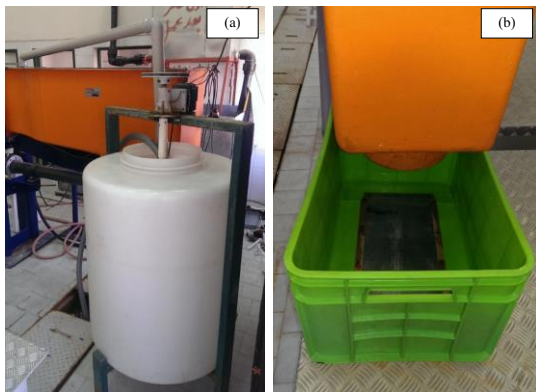
Figure 4. a) Density current production tank; b) material separating filter
