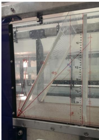
Figure 12. Selected angles of obstacle installation beyond 90°
