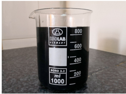
Fig. 6. A view of the prepared MWCNT-oil nanofluid with 0.2 wt%.
