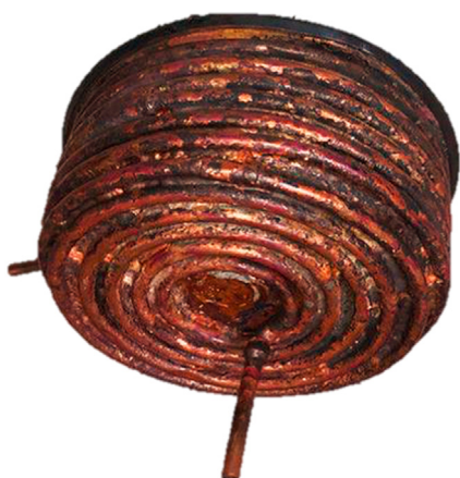
Fig. 3. A view of the cooking vessel along with the helical coil.
