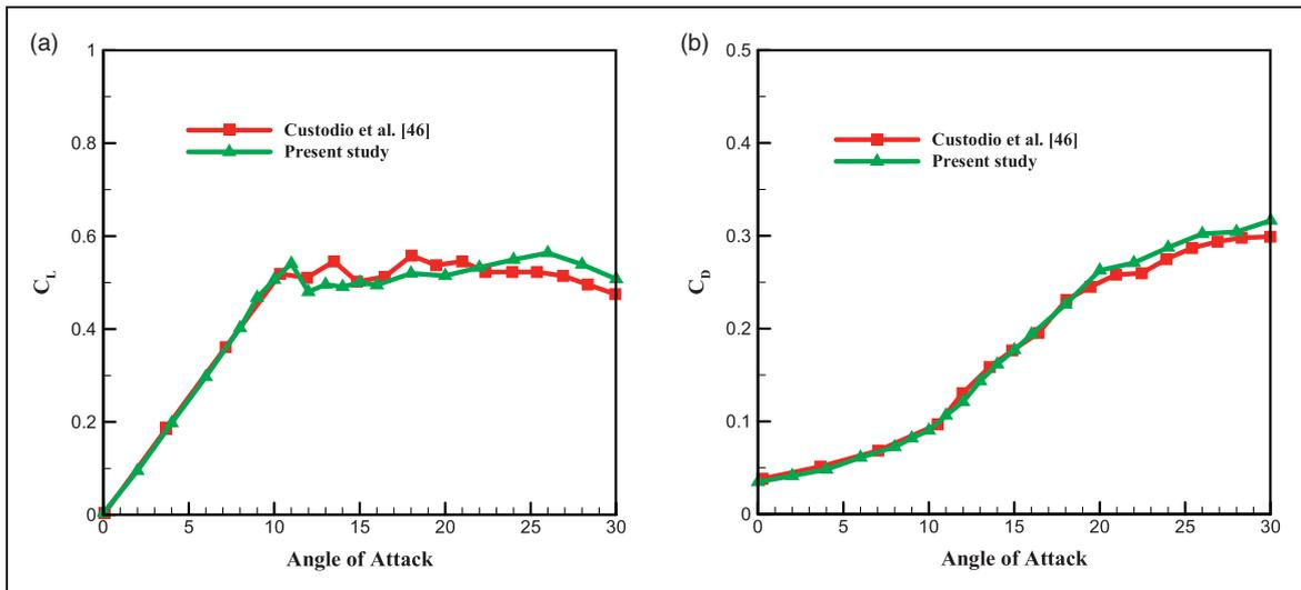
**Figure 6.** Comparison between aerodynamic coefficients of this study and those of Custodio et al.<sup>46</sup> (a) lift coefficient, and (b) drag coefficient versus angle of attack.
