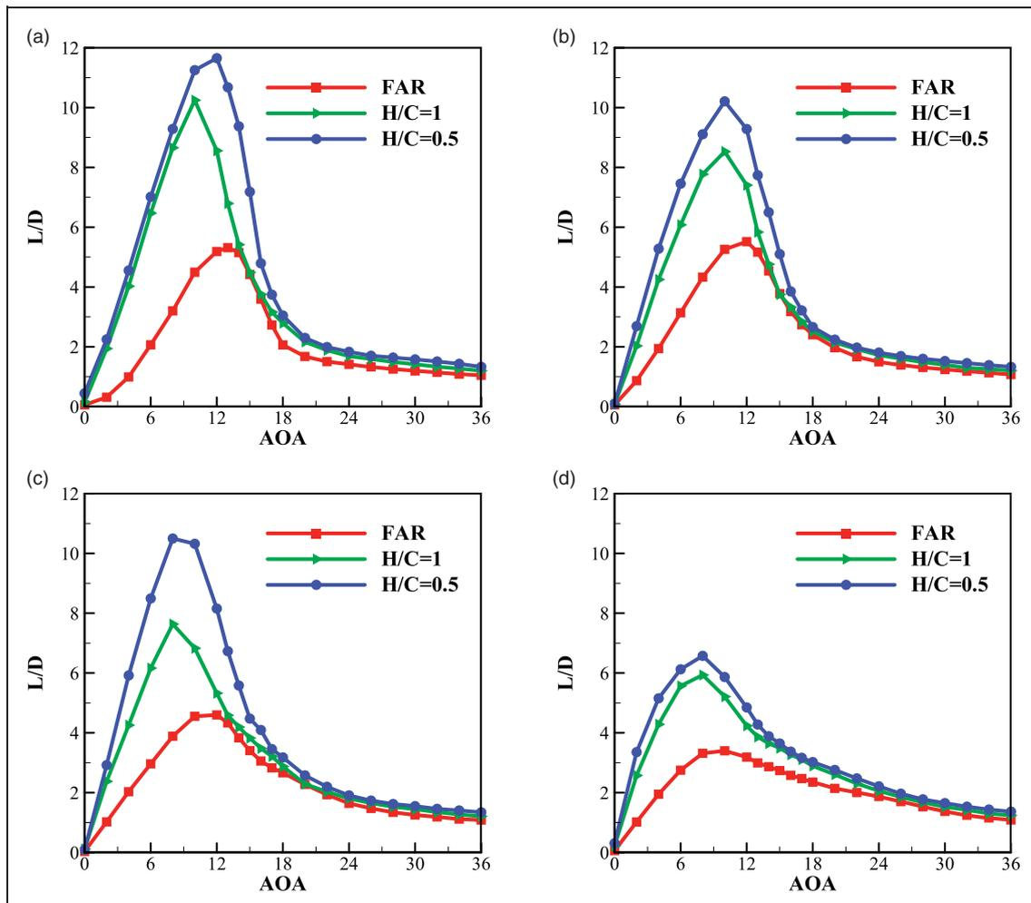
**Figure 12.** Variation of lift to drag ratio with angle of attack for different distances to ground (a) baseline (b) 4S (c) 4M (d) 4L.
