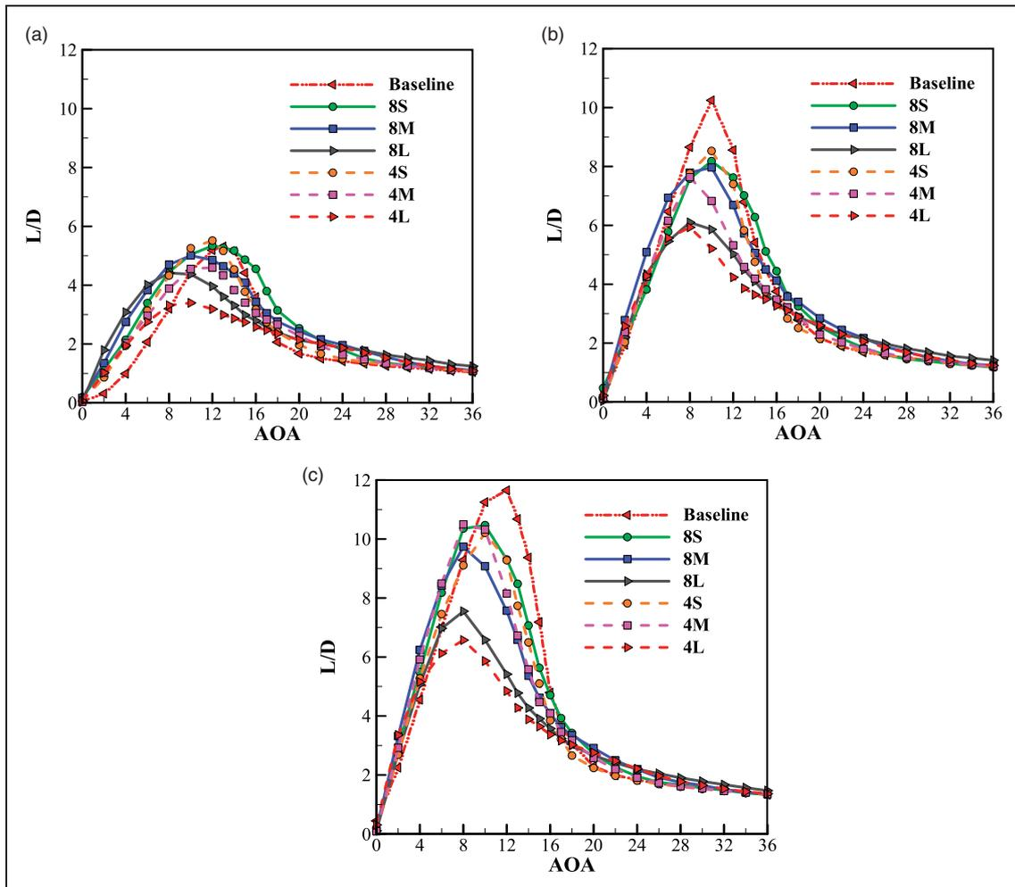
**Figure 14.** Variation of lift to drag ratio with angle of attack for different wings (a)  $H/C = \infty$  (b)  $H/C = 1$  (c)  $H/C = 0.5$ .
