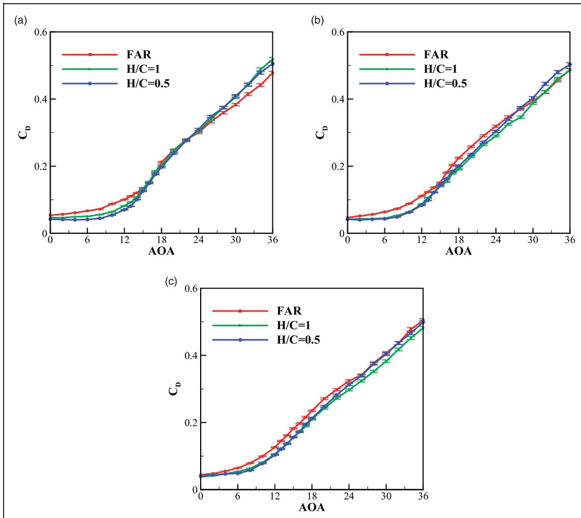
**Figure 10.** Variation of drag coefficient with angle of attack for different distances to ground (a) 8S (b) 8M (c) 8L.
