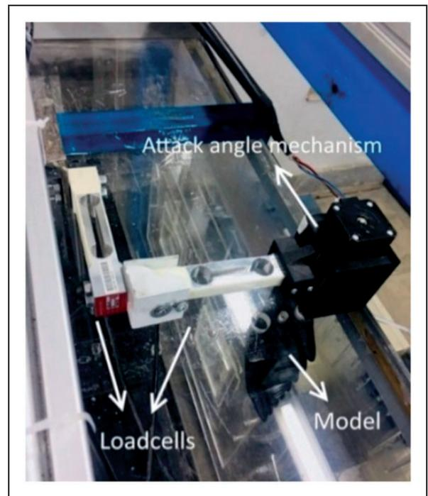
Figure 3. Designed and manufactured setups for load cells and attack angle adjustment.
