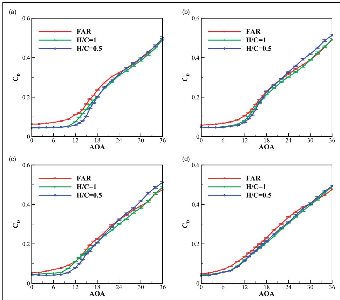
**Figure 9.** Variation of drag coefficient with angle of attack for different distances to ground (a) baseline (b) 4S (c) 4M (d) 4L.
