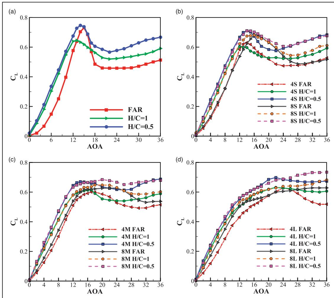
**Figure 7.** Variation of lift coefficient with angle of attack for different distances to ground (a) baseline (b) 4S and 8S (c) 4M and 8M (d) 4L and 8L.
