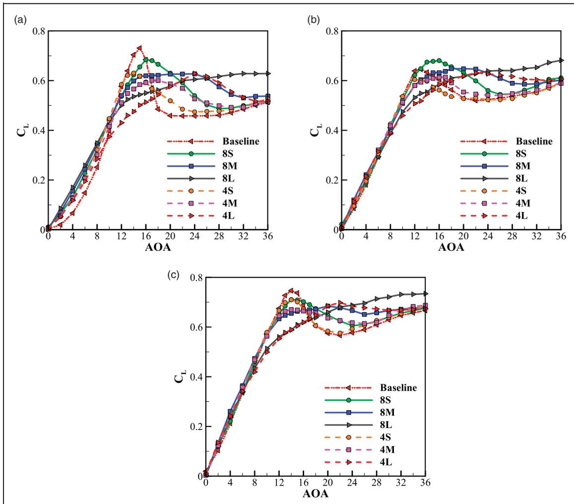
**Figure 8.** Variation of lift coefficient with angle of attack for different wings (a)  $H/C=\infty$  (b)  $H/C=1$  (c)  $H/C=0.5$ .
