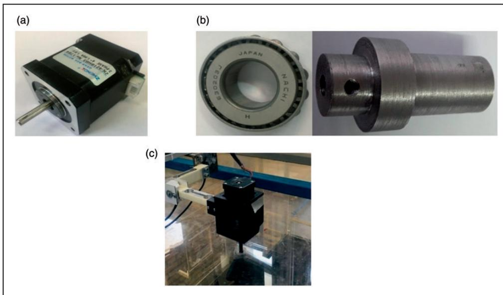
**Figure 4.** Views of Angle of attack mechanism; (a) stepper motor, (b) radial roller bearing, and (c) shield.
