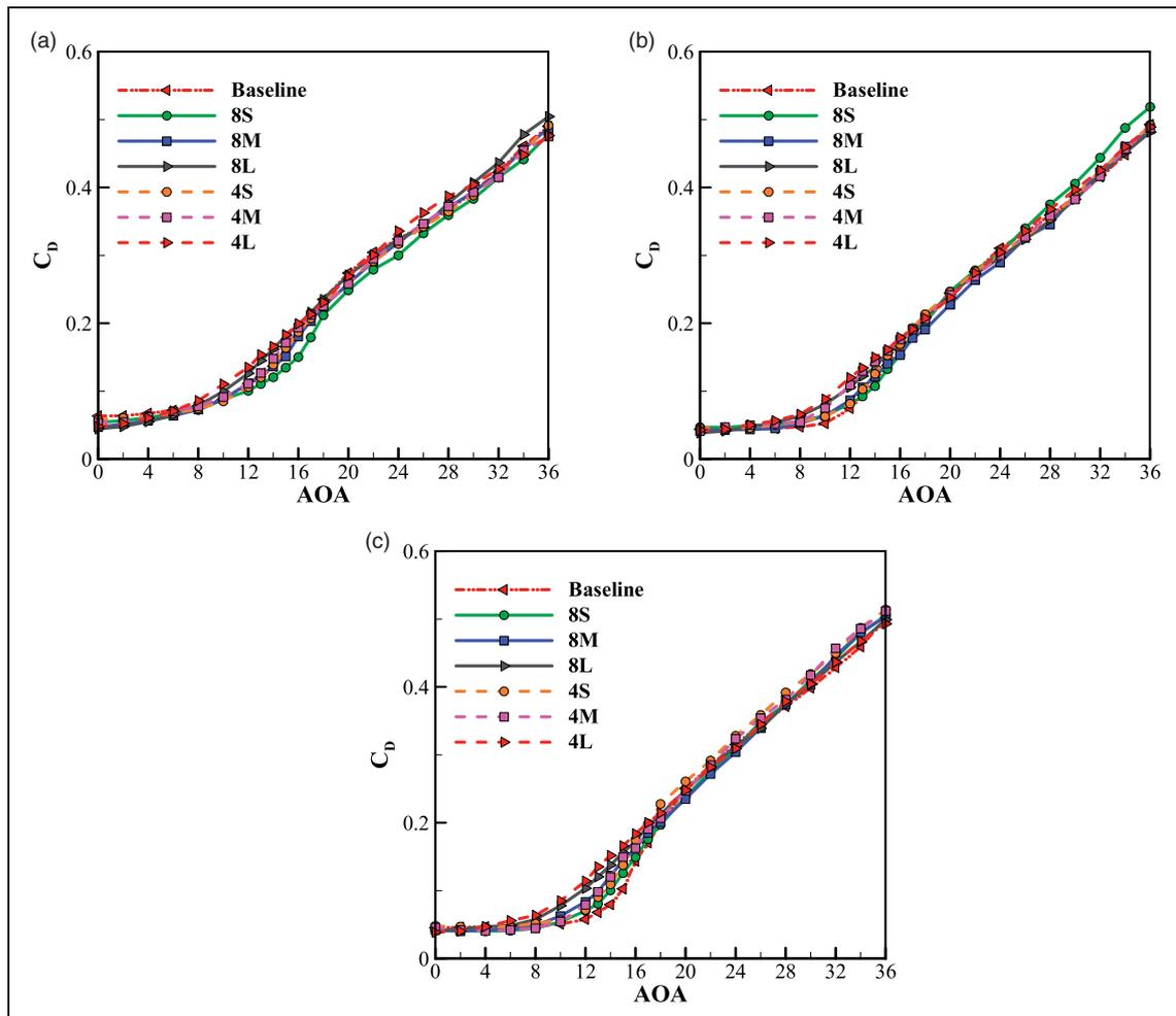
**Figure 11.** Variation of drag coefficient with angle of attack for different wings (a) H/C= $\infty$  (b) H/C = 1 (c) H/C = 0.5.
