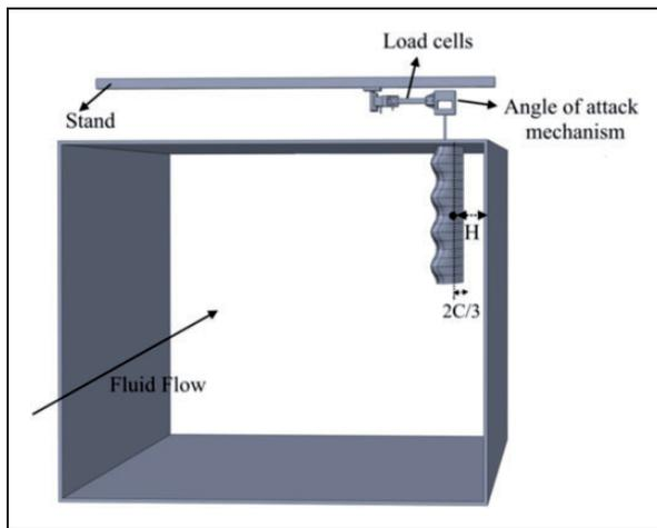
Figure 2. Schematic of the wing inside the wind tunnel.
