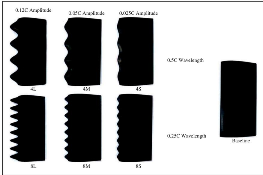
Figure 1. Manufactured wings.
