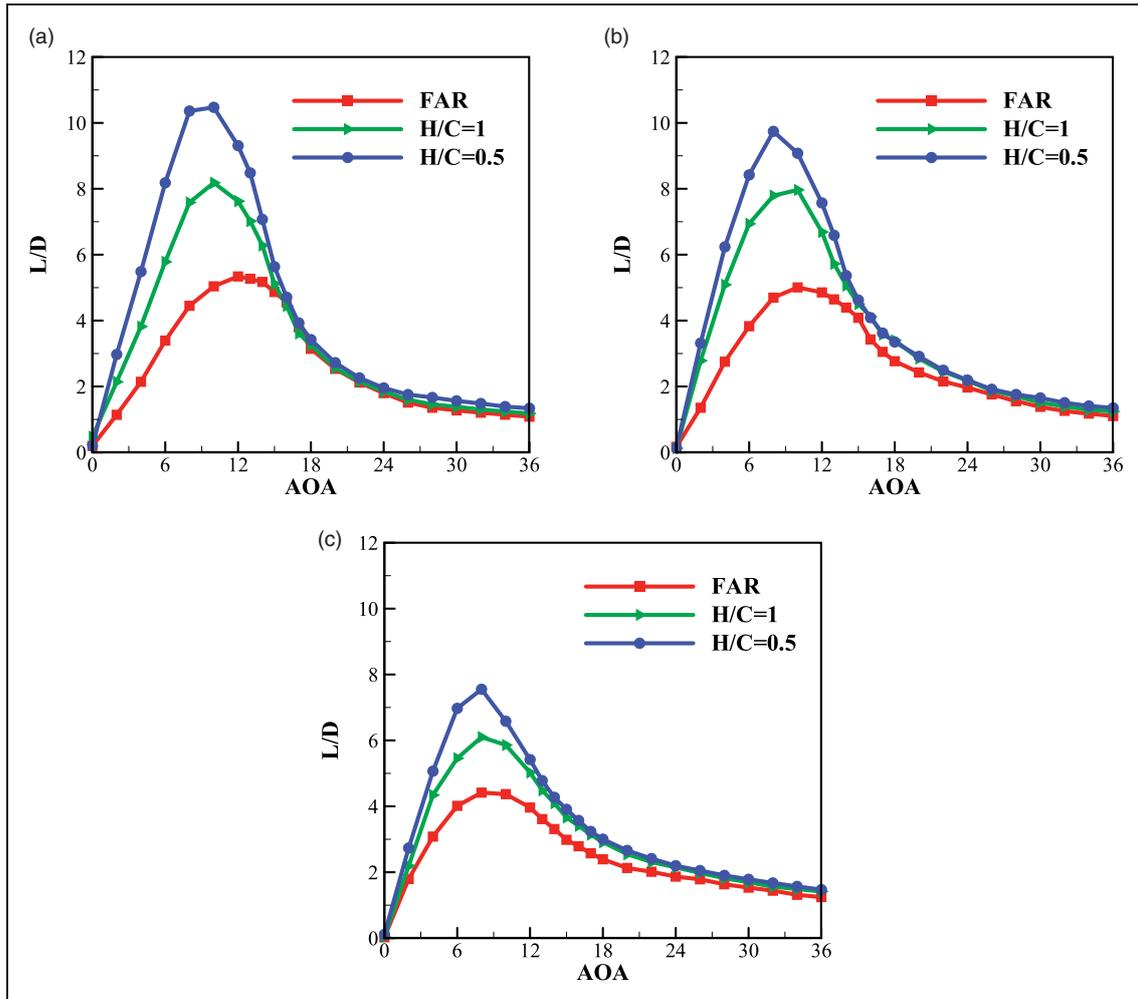
**Figure 13.** Variation of lift to drag ratio with angle of attack for different distances to ground (a) 8S (b) 8M (c) 8L.
