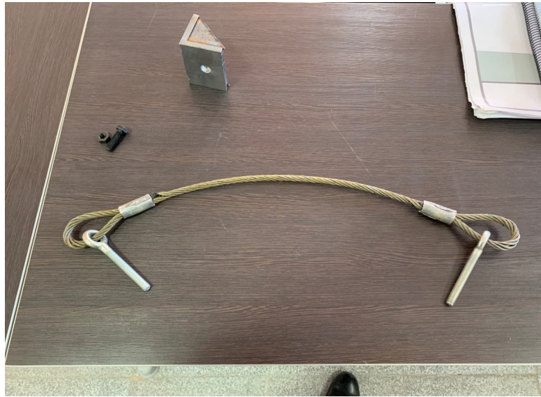
Figure 7: Woven cable around the connection tool to create the pre-tension force.
