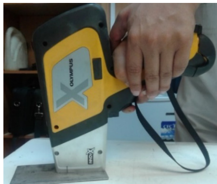
Fig. 2. Chemical composition determination using XRF test.
