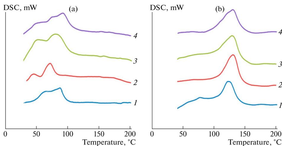
**Fig. 2.** DSC thermograms of (1) PE blend and PE/nanocomposites containing (2) MWCNT<sub>20–30 nm</sub> (0.74 wt %), (3) MWCNT<sub>30–50 nm</sub> (0.80 wt %), (4) graphene (0.30 wt %) obtained using N/Z/MMAO binary system: (a) S<sub>1</sub>, (b) S<sub>2</sub>.
