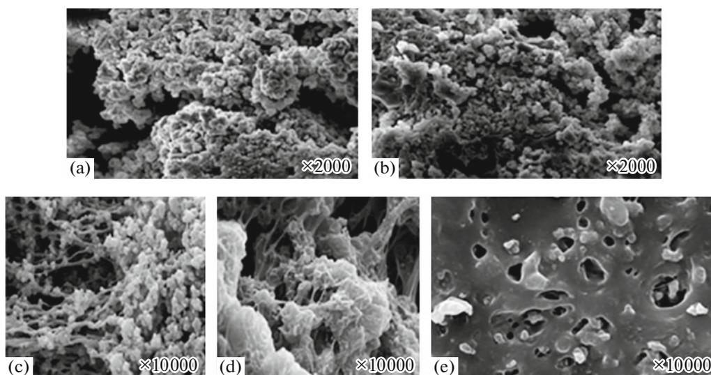
**Fig. 4.** SEM images of polyethylene blend prepared using N/Z/MMAO binary system of catalysts: (a)  $S_1$  (1 bar, 0°C), (b)  $S_1$  (4 bars, 0°C), (c)  $S_2$  (2 bars, 0°C), (d)  $S_2$  (4 bars, 0°C), and (e)  $S_2$  (2 bars, 30°C).
