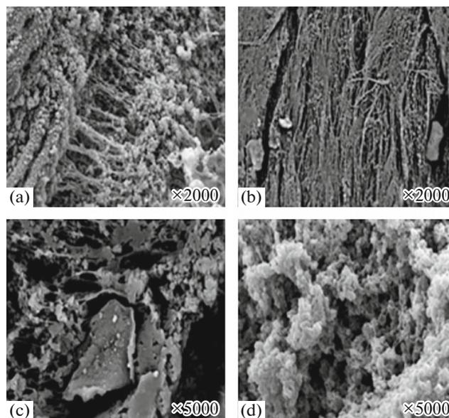
**Fig. 6.** SEM images of (a) polyethylene blend, and PE/nanocomposites containing (b) MWCNT<sub>20-30 nm</sub> (1.31 wt %), (c) MWCNT<sub>30-50 nm</sub> (0.97 wt %), (d) graphene (0.32 wt %), produced by  $S_2$  catalytic system.
