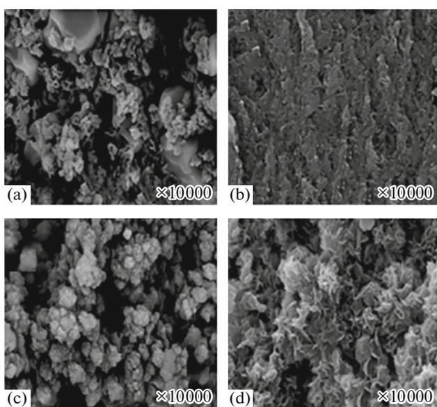
**Fig. 5.** SEM images of (a) polyethylene blend, and PE/nanocomposites containing (b) MWCNT<sub>20-30 nm</sub> (0.74 wt %), (c) MWCNT<sub>30-50 nm</sub> (0.80 wt %), (d) graphene (0.30 wt %), prepared by  $S_1$  catalytic system.
