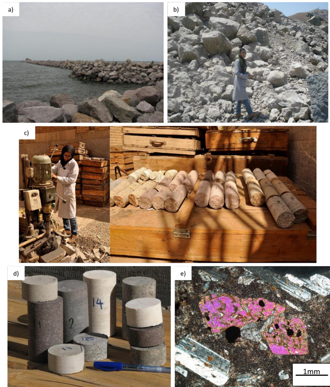
Figure 2- a) Sampling at one of the arms of the breakwater. b) Sampling at Isargaran Quarry. c) Coring of rock samples. d) Samples prepared for different experiments. e) Thin section of sample 2 (2.5X enlarged).
