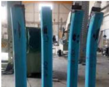
**Fig. 14.** Failing mode of specimens filled with plain concrete.
