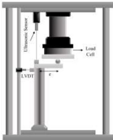
Fig. 10. schematic loading system.
