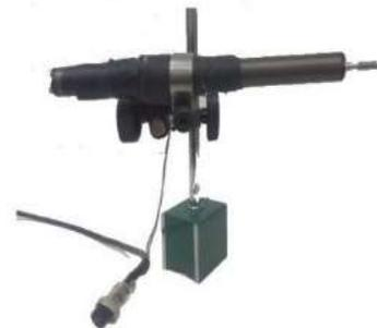
**Fig. 8.** electro mechanical LVDT
