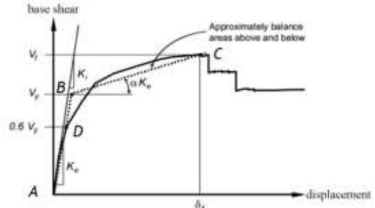
Fig. 3. Simplified diagram of force-displacement for  $\alpha > 0$  [29].
