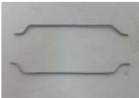
**Fig. 2.** Steel fibers used in concrete.
