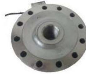
**Fig. 6.** 50 tonf weight load cell.
