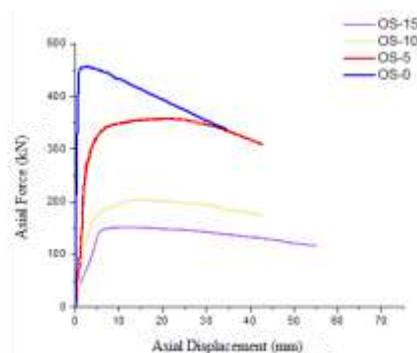
**Fig. 15.** Load-axial displacement diagrams of specimens filled with fiber reinforced concrete.
