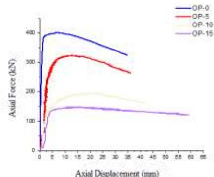
Fig. 12. Load-axial displacement diagrams of specimens filled with plain concrete.
