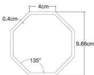
**Fig. 3.** Nominal dimensions of column section.
