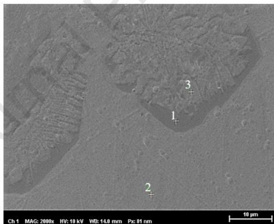
Fig. 4. Chemical composition analysis measured by EDS for the ingot with 1204 °C forging temperature (a) Matrix, (b) White phase.
