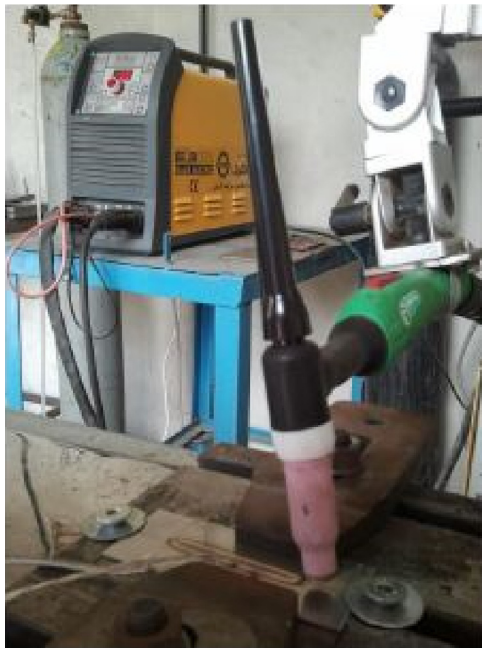
Fig. 2. PSQ 250 AC/DC (GAAM-Co, Iran) welding machine and welding torch.
