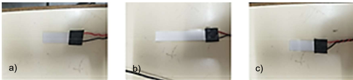
Figure 7 – PVDF piezoelectric devices to be used as fringes: a) device A; b) device B; c) device C.
