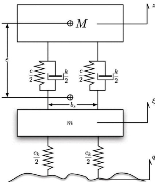
Fig. 8. The model of passive vehicle suspension [52].
