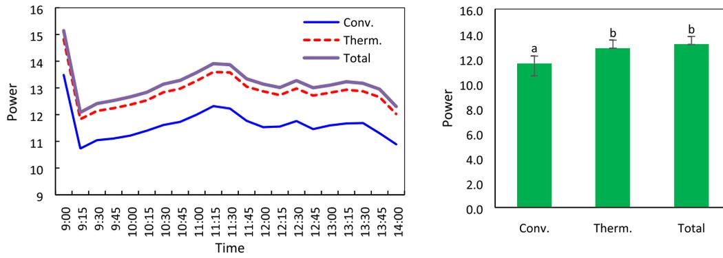
Fig. 4. Variations in the output power of the solar panel under normal operating conditions and the one using a thermoelectric module.
