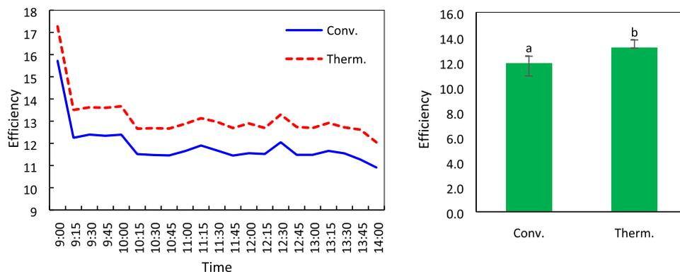
Fig. 5. Comparison of changes in solar panel surface efficiency under normal operating conditions and when using a thermoelectric module.
