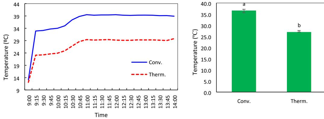
Fig. 3. Comparing surface temperature variations of the solar panel under normal operating conditions and when a thermoelectric module is used.
