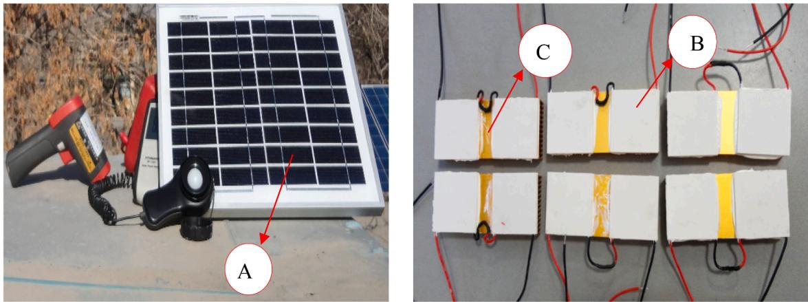
Fig. 1. The system presented in this study: A) Solar panel, B) Thermoelectric module, C) Heat sink.
