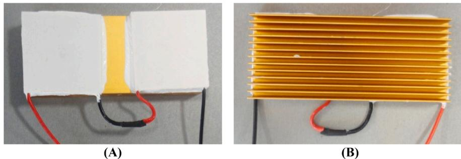
Fig. 2. A) Thermoelectric module, B) Anodized heat sink.
