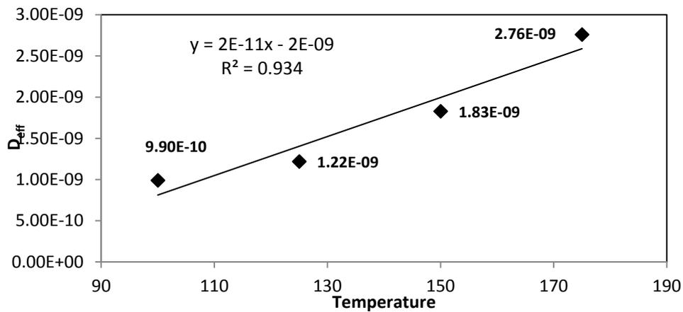
Fig. 5. Effect of drying temperature on the effective moisture diffusivity in lemon slices.
