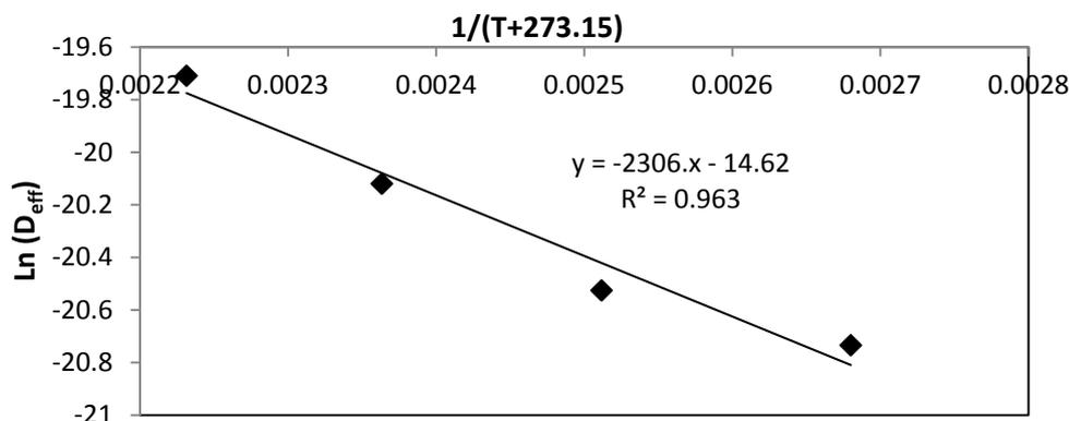
Fig.6. Influence of drying temperature on the effective diffusivity.
