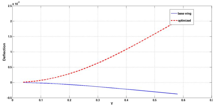
Figure 4. deflection distribution across wing span
