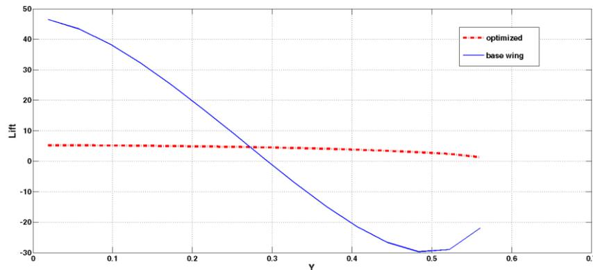
Figure 3. Lift distribution according to wing span
