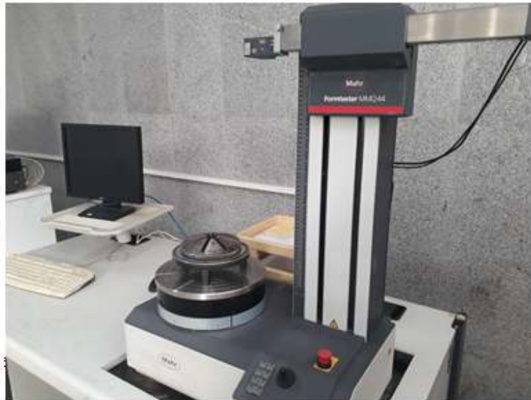
Fig. 2. The Formtester used for measuring dimensional and geometric specifications of cylinder liner. All dimensional and geometric specifications of the surface were evaluated with average values of five evaluation tests. The data were analyzed using descriptive statistics such as mean (M),
