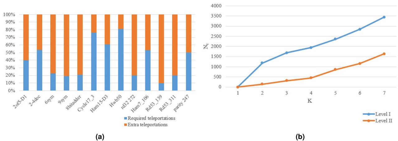
Figure 5. (a) Percentage of required number of teleportations to extra teleportations on Circuits 1 to 15. (b) The effect of the number of units on number of communications of Level I and II on Circuit Hwb50.
