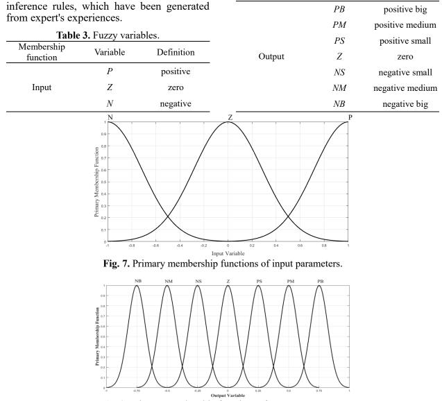
Fig. 8. Primary membership functions of output parameters.
