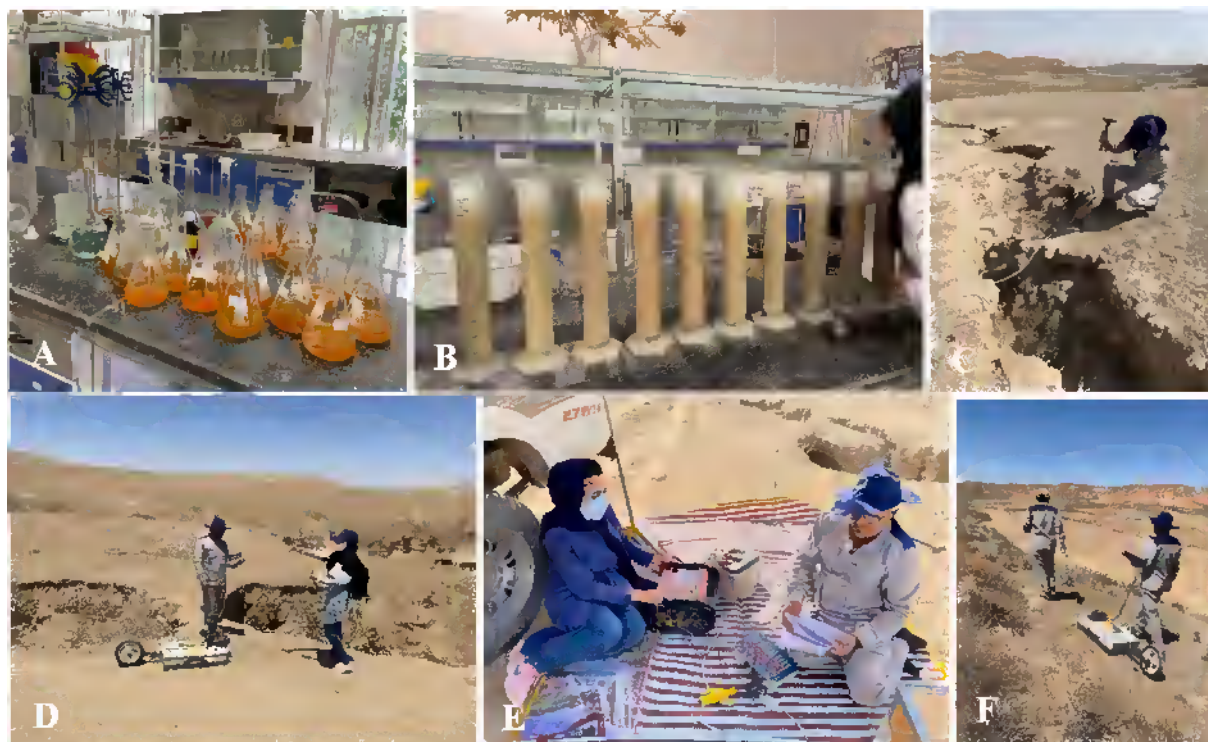
Fig. 5. Illustration of the laboratory and field measurements made at the two study sites. A = chemical analysis of soil samples, B = soil textural analysis, C = GPR at site 2, D = ERT at site 2, E = GPR at site 1, and F = ERT at site 1.
