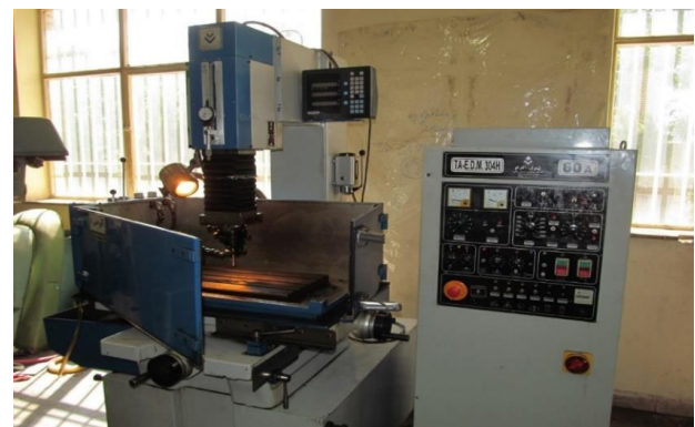
Figure 2 Azerakhsh-304H EDM machine used
