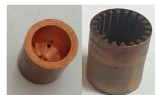
Fig. 5 Used preform in flow-forming and flow-formed gear
