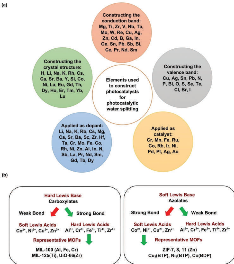
Figure 8. (a) elements used in different parts of photocatalysts for water splitting. (b) strategies to construct stable MOFs guided by HSAB theory. Reprinted with permission from Ref. [186] copyright 2018 advanced materia.
