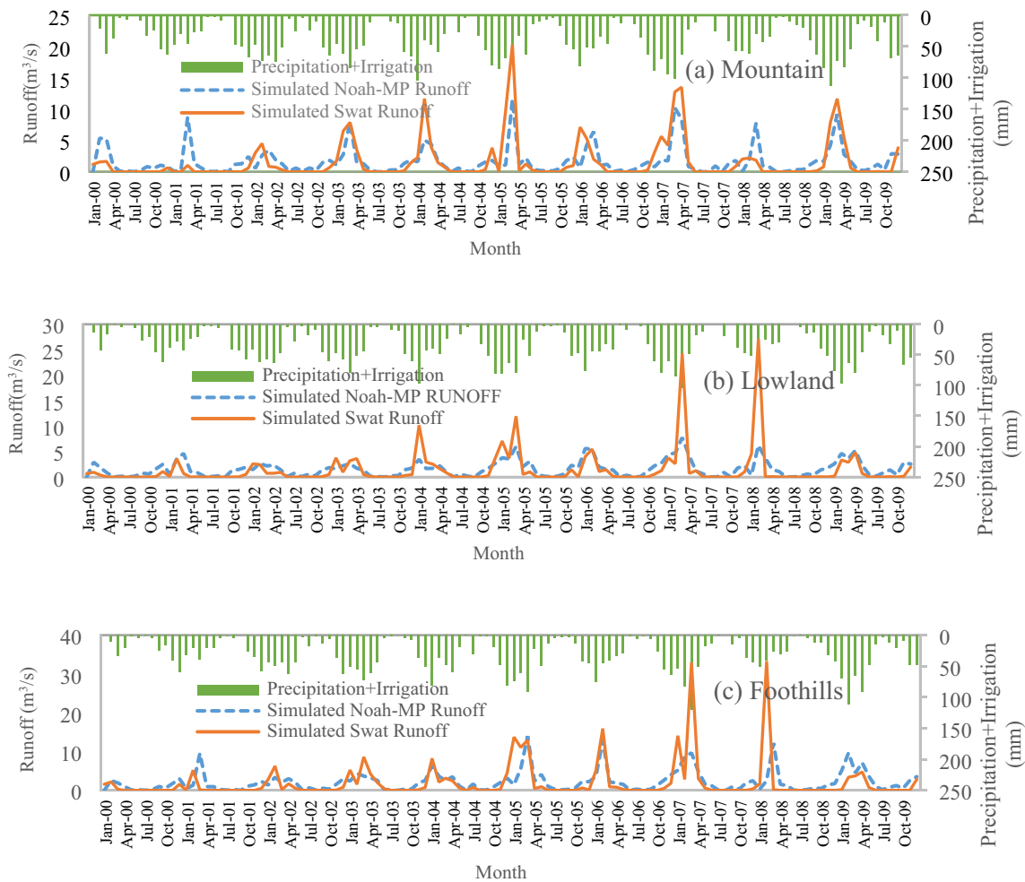
Fig. 3 Simulated monthly runoff by Noah-MP and SWAT model and sum of irrigation and precipitation in a mountain, b lowland, and c foothills
