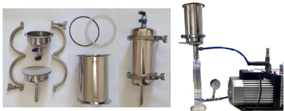
Fig. 1 The vacuum pump and the main components of Büchner funnel used in vacuum filtration system
