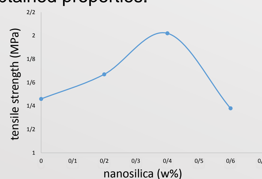
Fig. 1: change in tensile strength of HMPUA with nanosilica (0, 0.2, 0.4 and 0.6 w%).
