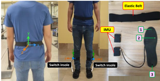
Figure 1. Components of the experiment setup and lower back IMU alignment. Numbers 1, 2 and 3 indicate the embedded switches
