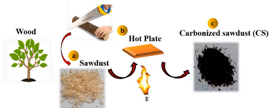
Fig. 3. Schematic of the carbonized sawdust (CS) preparation process: (a) Sawdust, (b) Carbonization at a surface temperature of 200 °C using a burner, (c) the CS.
