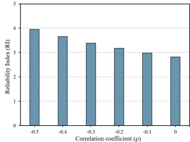
Figure 7. RI values versus correlation coefficient between cohesion and friction angle.
