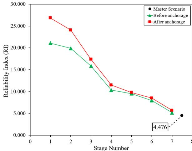
Figure 6. Variation of RI with excavation stages before and after anchorage due to internal friction angle variability of all layers with COV<sub>φ</sub>=0.2.
