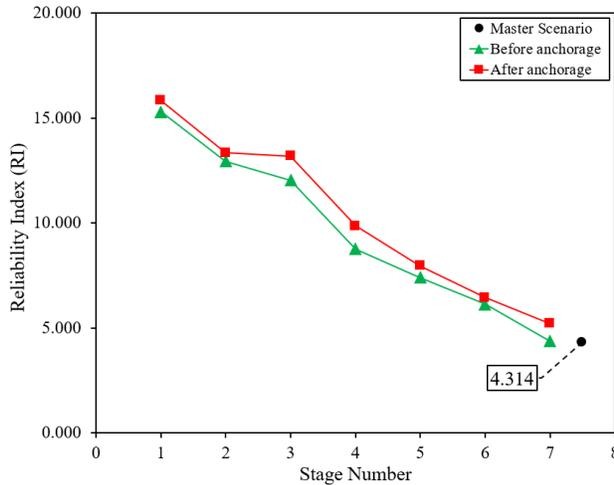
Figure 5. Variation of RI with excavation stages before and after anchorage due to cohesion variability of all layers with COV<sub>c</sub>=0.5.
