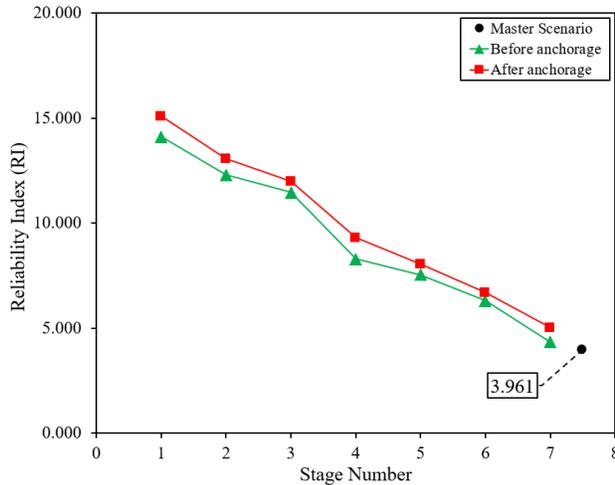
Figure 8. Variation of RI with excavation stages before and after anchorage when  $COVC = 50$ ,  $COV_{\phi} = 50$ , and  $\rho = -0.5$ .
