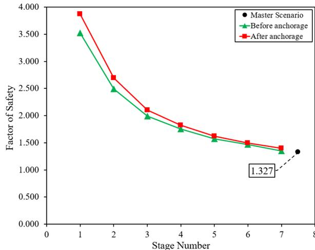
Figure 2. Variation of deterministic FS with various excavation stages.
