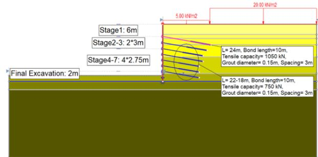
Figure 1. Numerical model with PAS parameters.
