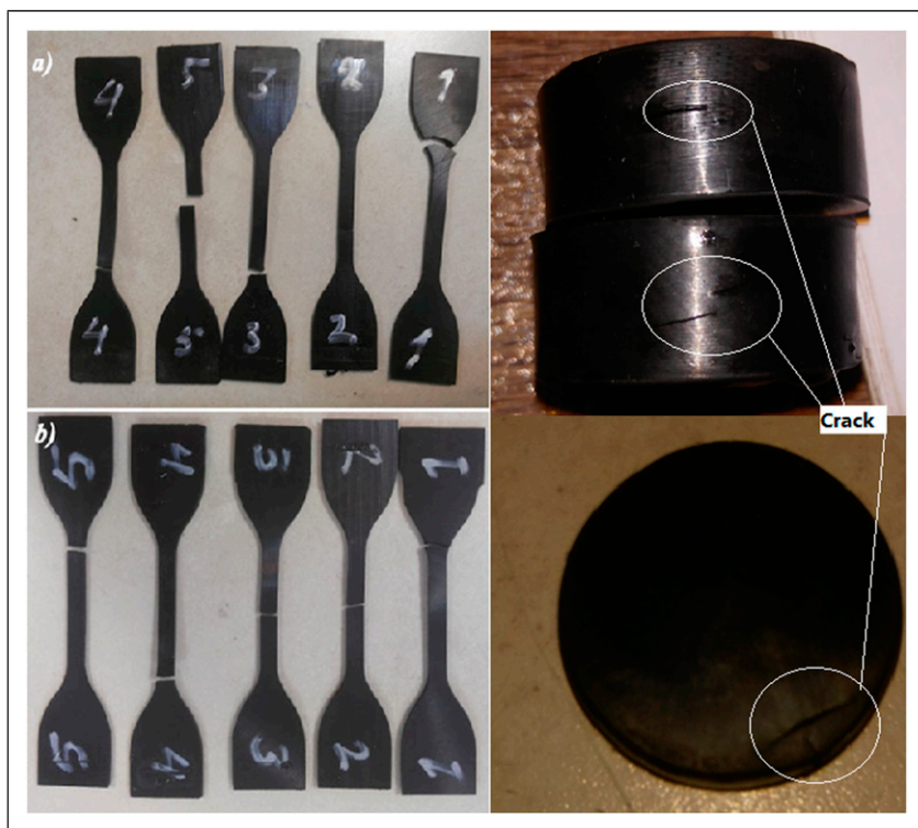
Figure 6. Macrography of tensile and compression set specimens of aged HNBR rubbers by a) Hc-A and b) Hc-B method.
