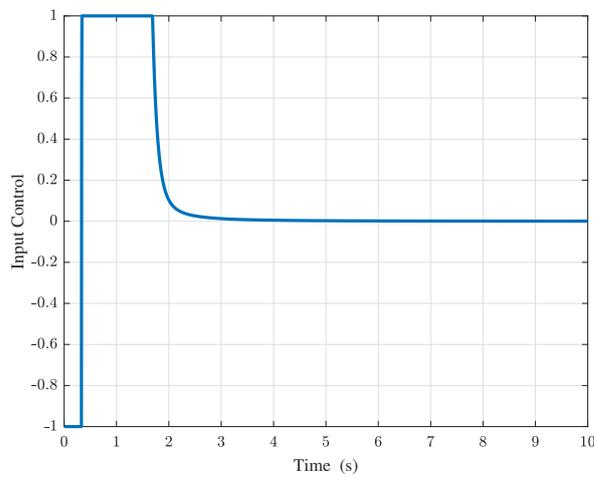
Figure 9. Input saturation control.
