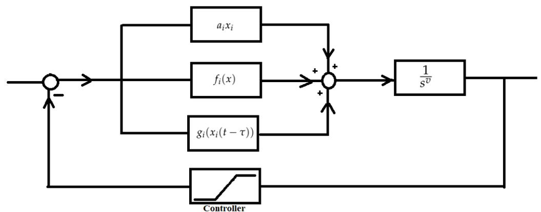
Figure 1. Block diagram of the FO delayed system subject to saturation control.
