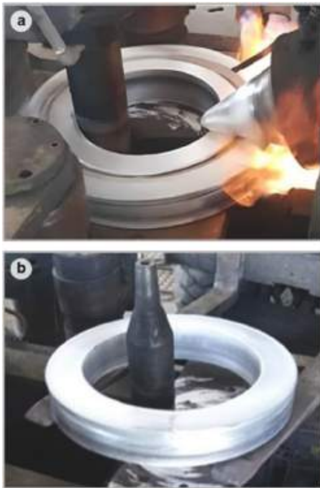
Fig. 3. (a) Ring rolled alloy in the final step of deformation, and (b) final product after cooling.
