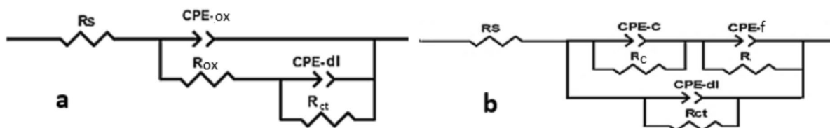
Fig. 10 The equivalent circuit used in modeling a 304 stainless substrates; b AlPO_4 coating in industrial H_2SO_4 solution
